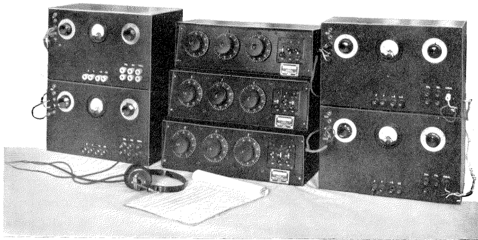
Fig. 5—Mixers and Pre-amplifiers at Heroes' Square.
