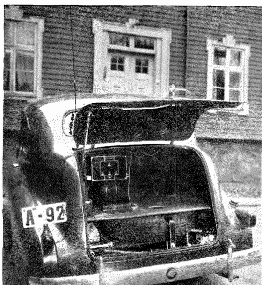
Fig. 7—Transmitter and Power Units in a Government Police Car.
