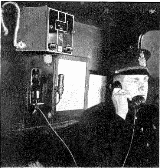
Fig. 5.B.—Receiver and Control Unit in Transport Car.
