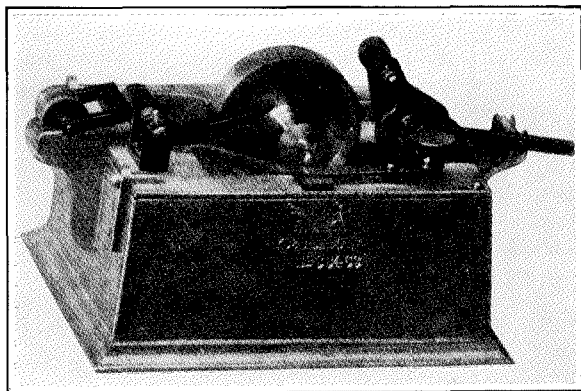
Figure 7—Gummer. (Machine for Gumming the Slip.)
