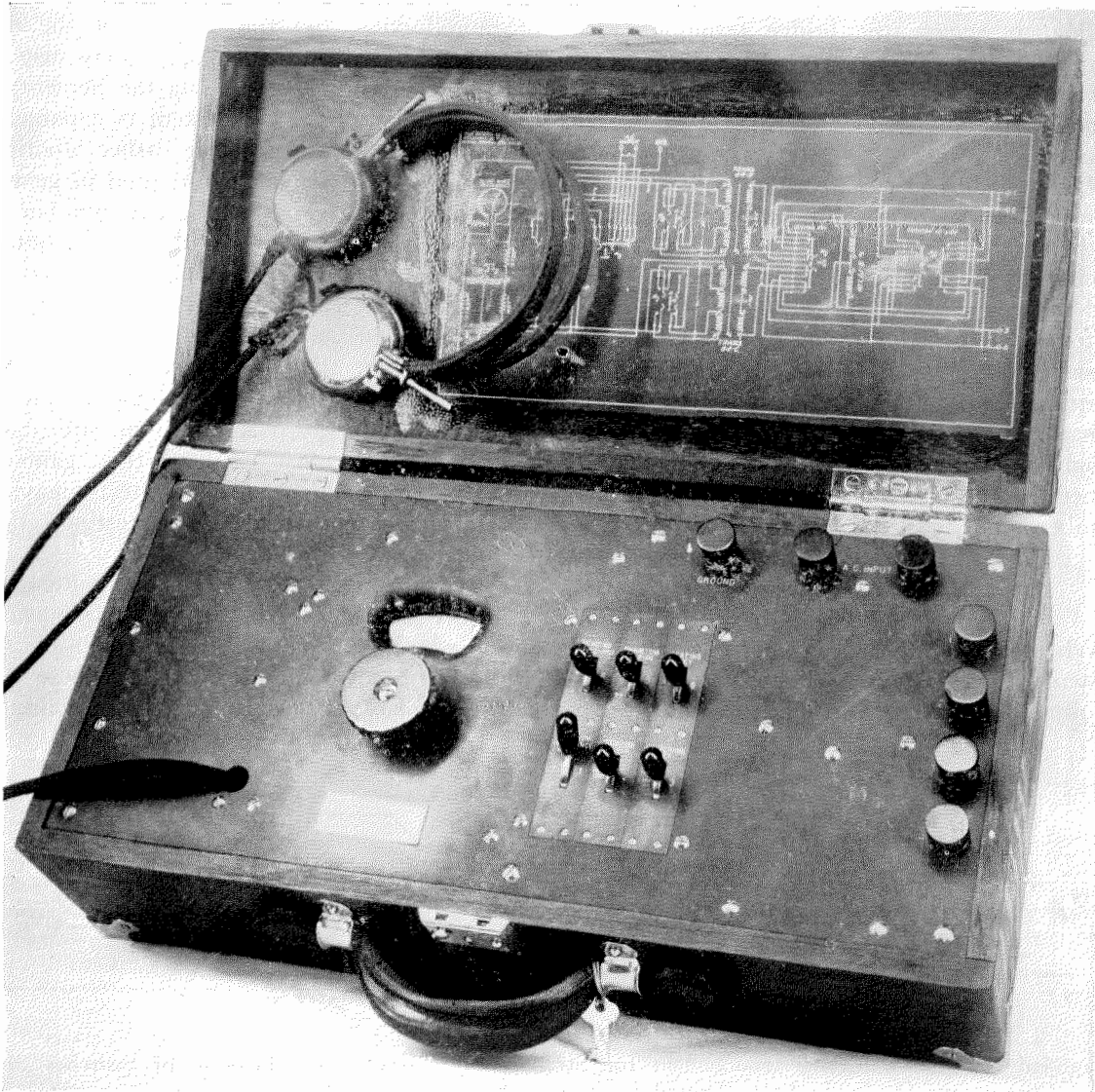
Figure 8—Crosstalk Measuring Set
