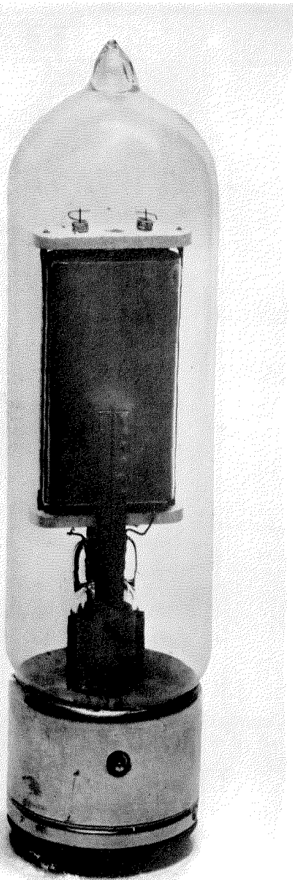
Figure 12—No. 211-A Vacuum Tube
