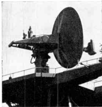
STABILIZED ANTENNA for the U.S. Navy's SPS-30 shipboard radar is actuated in roll and pitch by a unique dual ball-screw drive. The precision, electro-formed organ-pipe scanner permits long-range, high-accuracy search and height-finding capability.
