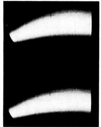
Fig. 4- Noise output of RWT R-B1 superheterodyne receiver without VA-99 preamplifier (top) and with VA-99 preamplifier (bottom).
