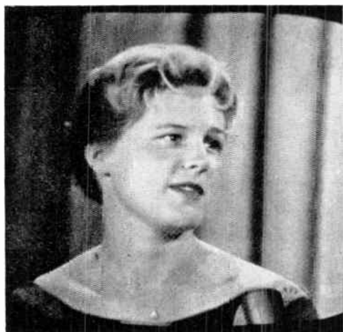
Fig. 33—Monochrome display of color picture after transmission as seven digit PCM.
