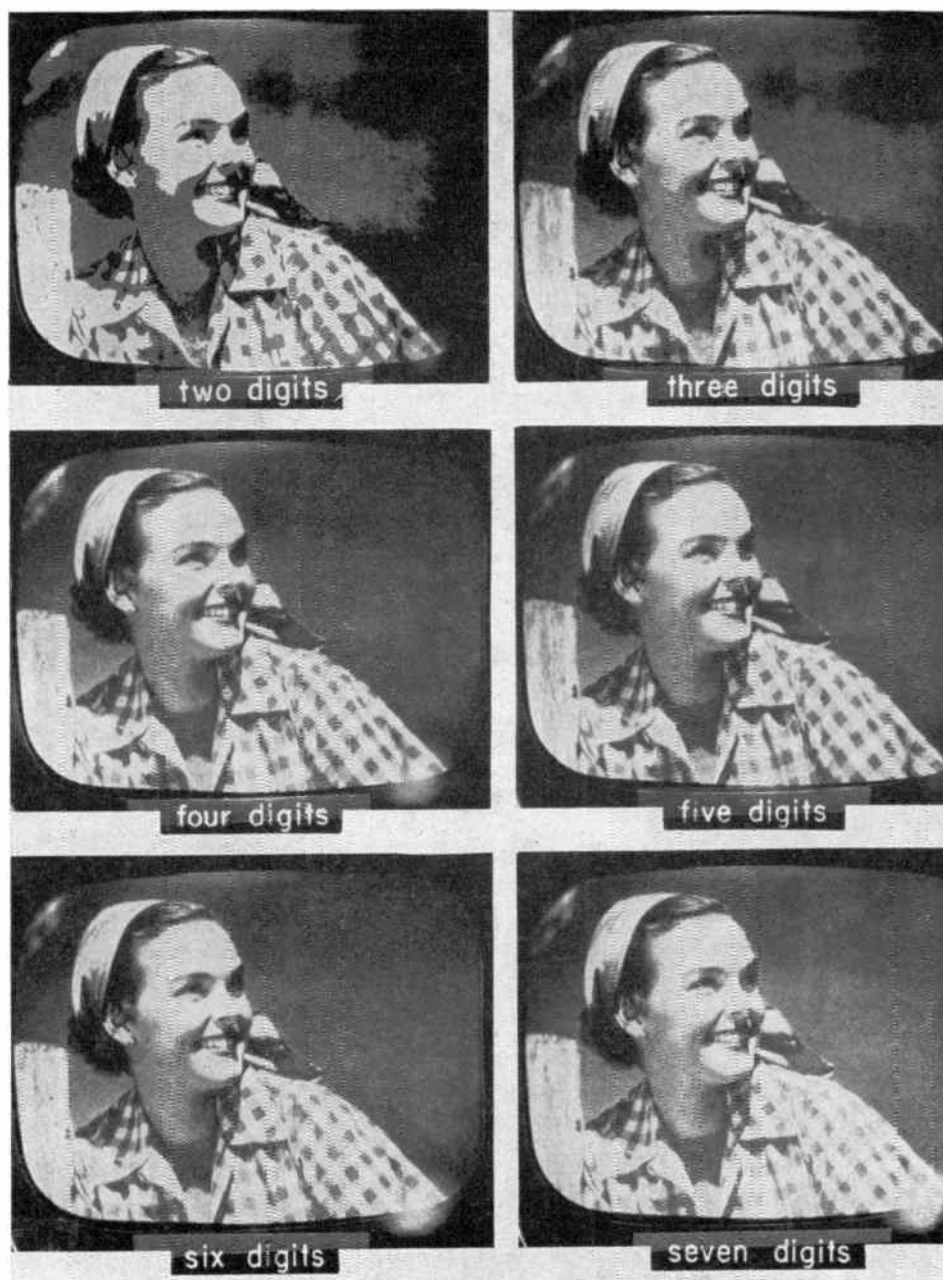
Fig. 32—TV picture showing the effect of adding one digit at a time, starting with two digits and ending at seven digits.
