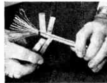
Shielding cables reduces magnetic radiation or pickup.
