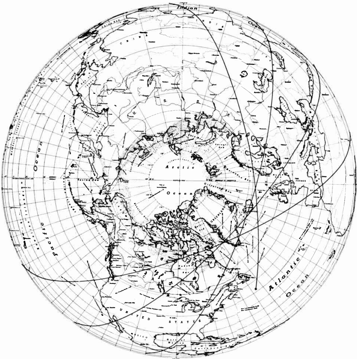
Fig. 1—Several orbits of an artificial earth satellite on an orthographic polar projection showing precessing due to earth's rotation.
