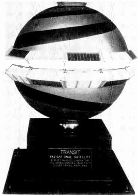
Fig. 4—TRANSIT satellite showing spiral slot antenna.
