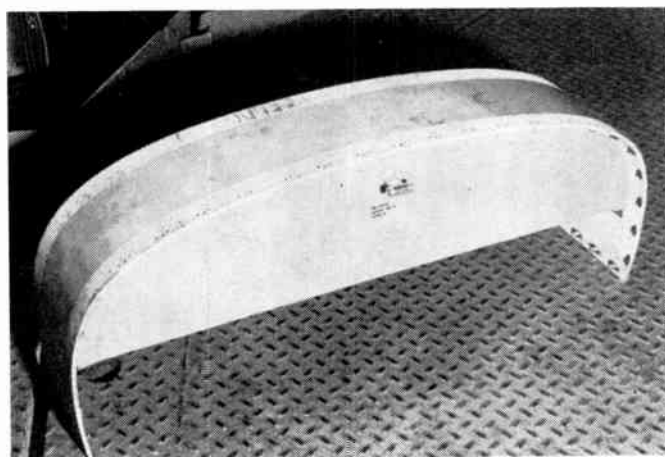
Fig. 4—Slot antenna used with SCORE satellite.
