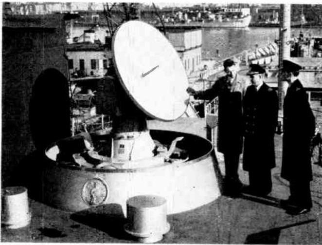
Fig. 1—Radio Sextant AN/SRN-4 (courtesy of Collins Radio Company). (Official U. S. Navy photograph.)
