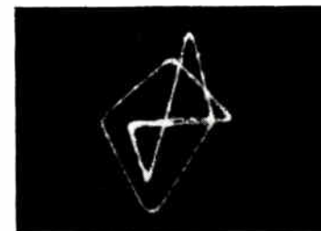
In research laboratory studies at Ramo-Wooldridge, electrically-charged particles are contained and supported in a vacuum by an alternating electric field
