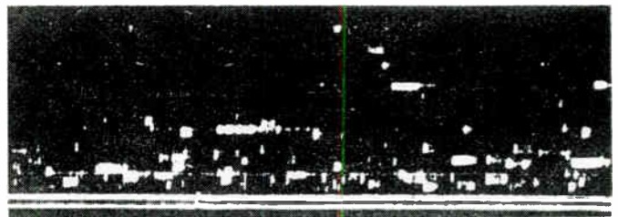
Fig. 1—Display of meteor activity on 23.1 mc at Stanford, Calif., at 0310, January, 1956. An array of 48 Yagi antennas was beamed north. The vertical range scale covers 1000 km, and the time scale covers 40 seconds reading from left to right. The peak transmitted power was 35 kw.
