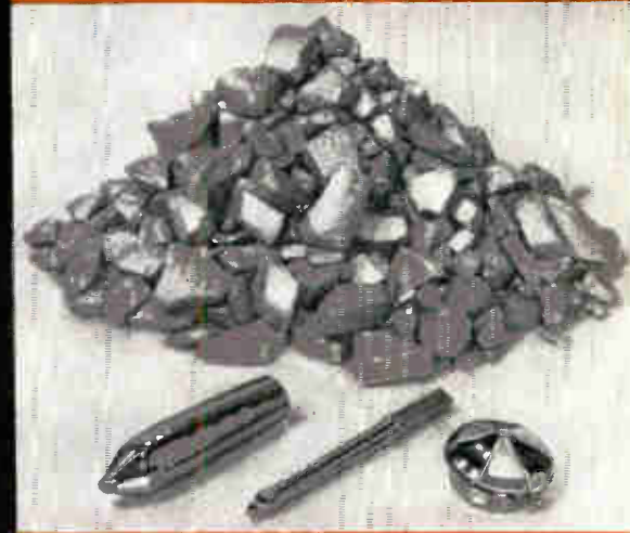
Three characterization crystals are grown from each lot — one for resistivity, type and lifetime determination, another for cleanliness a third for boron content.
