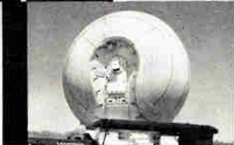
Two tracking-radar antennas, housed in radomes, take over. One feeds target azimuth, elevation, range data to computers; other tracks Hercules.
