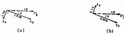
Fig. 2—Phasor diagrams for 10-db short-slot couplers: (a) sidewall coupler, (b) topwall coupler.
