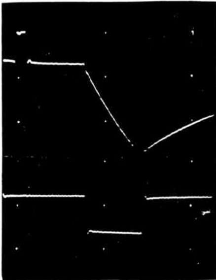
Fig. 10—Upper: record of membrane potential response to a step of current density, preceded by response to test pulse applied to input of microelectrode amplifier. Lower: record of current pulse of 250- \mu sec duration.
