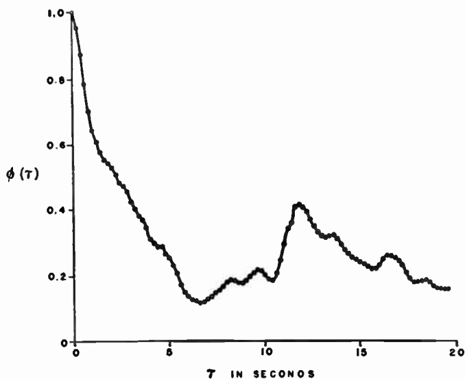
Fig. 16—Normalized autocorrelation function \phi(\tau) computed from 71 seconds of recorded unrest of experiment no. 5.
