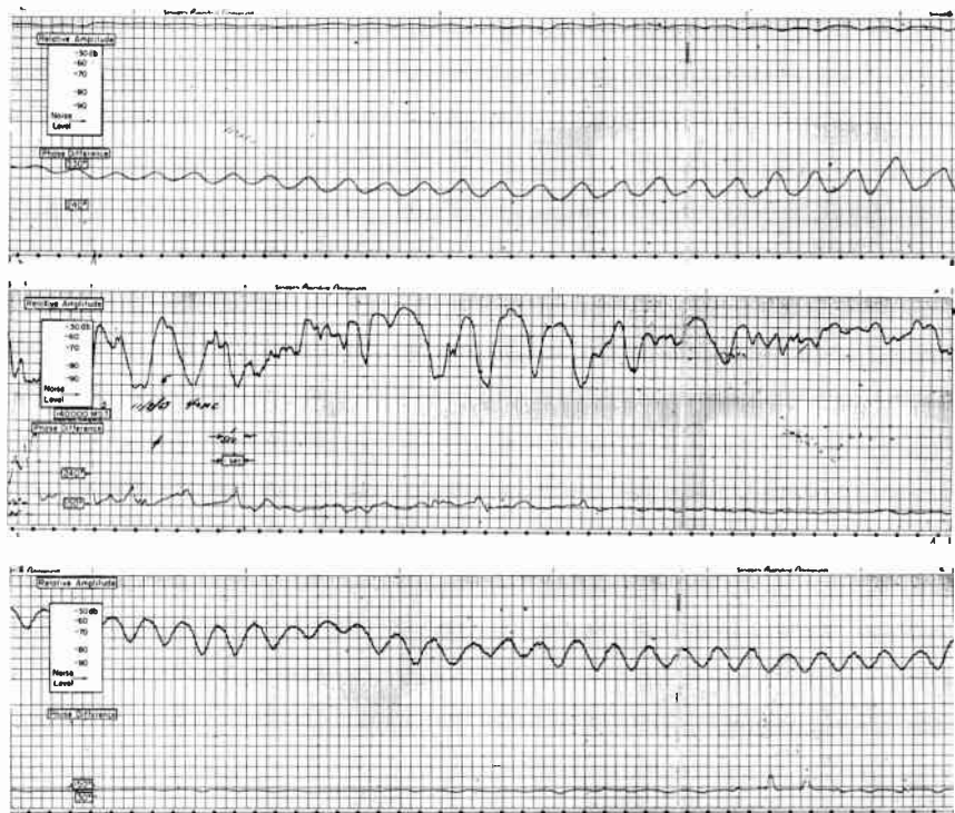
Fig. 1—Sample of relative phase of 40-mc signals received on two antennas spaced 1000 feet (bottom traces on each section) and relative amplitude of signal from one antenna (upper traces). First section represents approximate time of nearest approach, second section, early part of passage (satellite approaching from NW), and third section, approaching end of passage.
