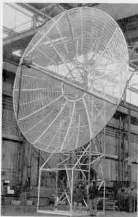
Above—A mobile antenna for use at frequencies between 200 and 4000 mc, has a 28-foot diameter reflector which is sectionalized for storage within its mounting tower. Retractable wheels in the tower can be used for towing.
