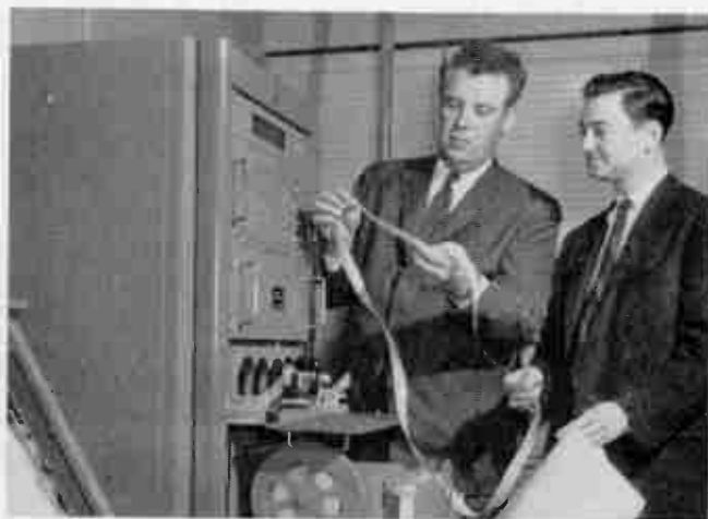
Above—The electronic spectroanalyzer determines the identity of chemicals by the quantity of infrared waves which are absorbed. Major units are a spectrophotometer, a recording device, a "library," and a high speed electronic computer. It is useful in medical electronics and nuclear radiation analysis.
