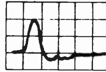
Fig. 16—Photograph of a clock generator pulse (abscissa 50 \mu sec per division and ordinate 12 v per division).
