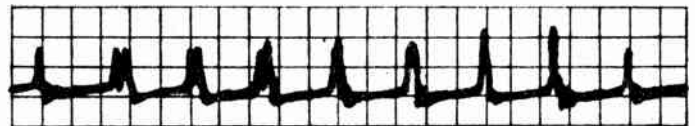
Fig. 20—Photograph of the vernier and clock pulses resistively added (corresponding to the stop measurement of Fig. 12).
