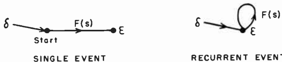
Fig. 10—Closing the feedback loop produces a recurrent process from the single-event diagram.
