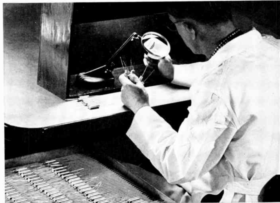
OIL-FILLED CAPACITORS are subjected to vacuum under elevated temperatures, then are individually examined to insure complete hermetic seal.
