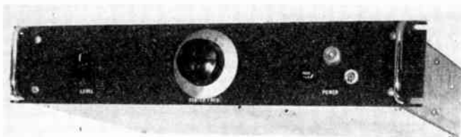
Fig. 4—SSB/FSK exciter accepts frequency shifted tone keying signals in the range 425 to 2465 cycles and converts them to 200 kc range. The 200 kc signals are applied, over coaxial cable, to radio frequency converter in transmitter proper.
