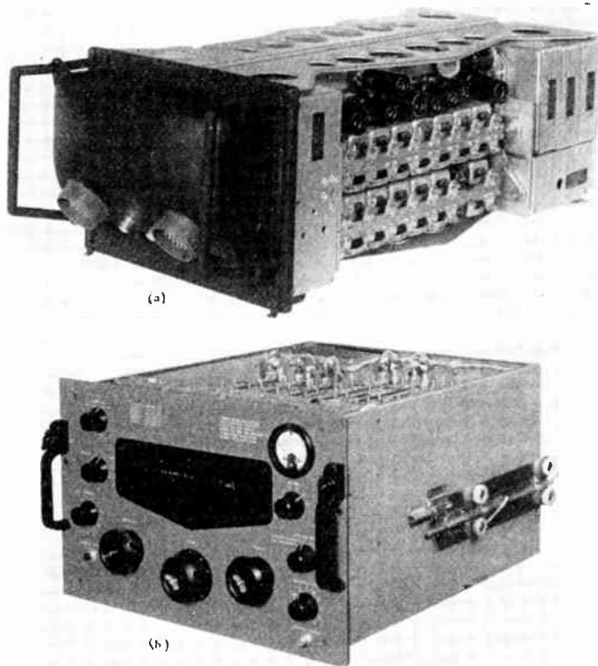
Fig. 1—(a) Aircraft SSB exciter with servo coupled mixer-multiplier. All units are plug-in module construction. (b) SSB ground station exciter drawer. All mixer-multipliers and oscillators are mechanically ganged to front gear plate.
