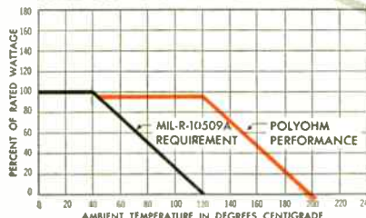
DERATING CURVE FOR HIGH AMBIENT TEMPERATURES
