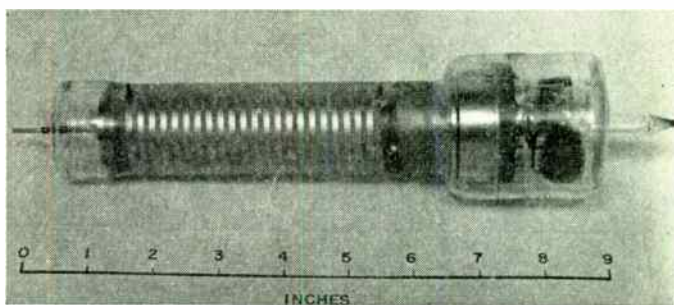
Fig. 8—Photograph of the 500–1,000 mc backward-wave oscillator used to measure the effect of velocity spread on the efficiency. The oscillator used a hollow electron beam placed close to the helix.
