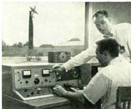
Electronics Research Engineer T. W. Hancock and Electronics Engineer Irving Alne discuss asymmetry in Super Constellation antenna pattern.
