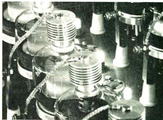
EXAMPLE OF HIGH POWER OUTPUT CAPABILITIES OF EIMAC TUBES IN TYPICAL PLATE PULSED RF AMPLIFIER OPERATION
