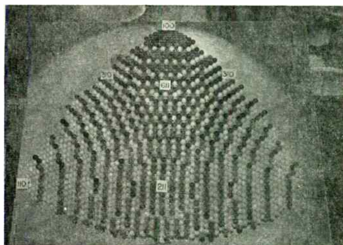
Fig. 5—"Marbles-for-atoms" model of a portion of a hemispherical tungsten field emitter tip with several crystal facets identified in correspondence with areas in emission pattern of Fig. 4.
