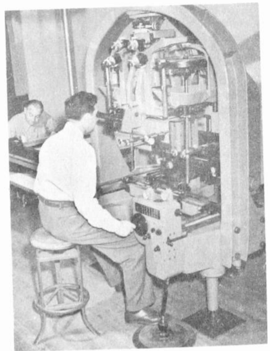
Fig. 7 A Wild Autograph, Model A-5. One of the most complex and precise photogrammetric instruments.
