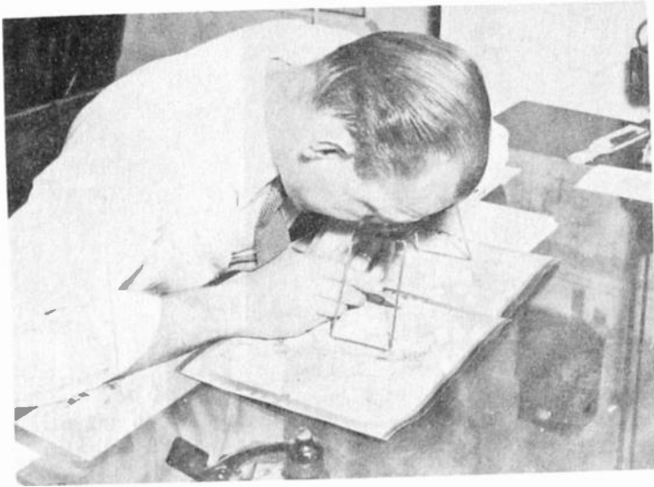
Fig. 4 Folding pocket stereoscope being used for study of aerial photographs.
