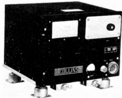
Fig. 10 Complete automatic antenna matching unit.
