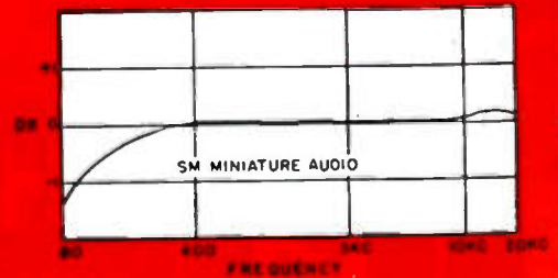
SM sub-miniature audio components, 7/16" x 1/2" x 7/16" height. Weight — .009 lbs.
