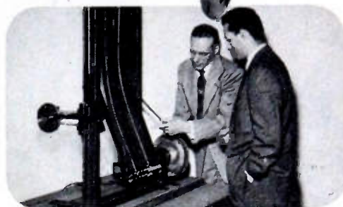
Remember this traffic-stopper of the 1952 IRE Show in Grand Central Palace? It's a torture test. Flexed well over 1,000,000 times, Waveflex flexible Waveguides gave no evidence of failure or loss of physical or electrical properties.
