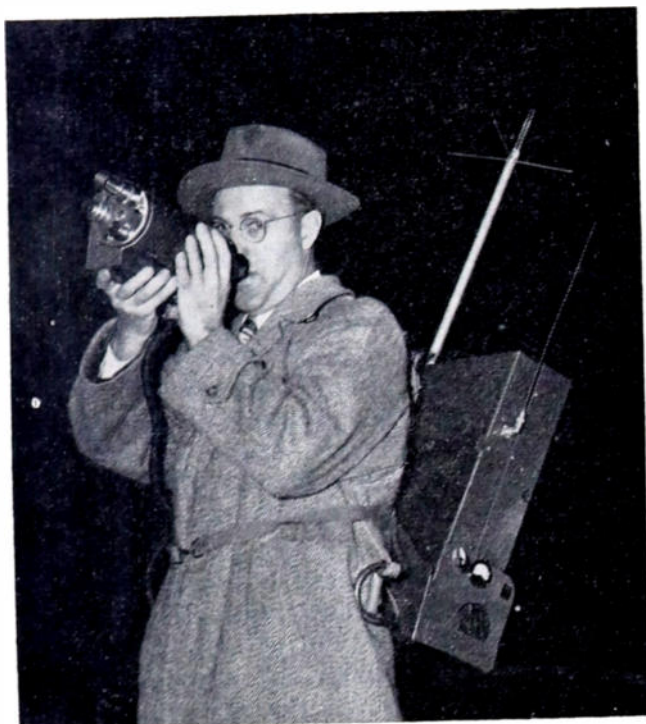
Fig. 9—Back-pack television transmitter receiver developed for use in picking up remote telecasts. The special vidicon camera is equipped with a view finder and lens turret. The receiver portion of the pack unit gives the operator constant contact with the control unit, which may be as far as a mile away (RCA).
