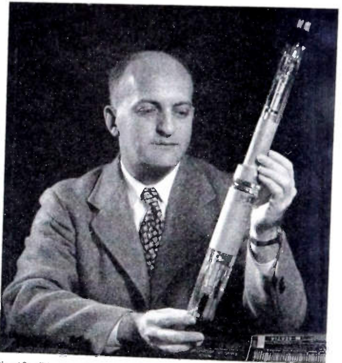
Fig. 19—The Graphechon, "visual memory tube," stores and amplifies weak but brief signal, such as oscilloscope traces or radar "pips" for as long as a minute (RCA).
