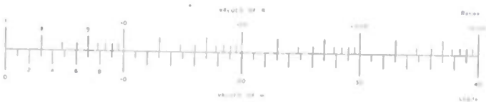
Fig. 1—Scales of actual relative magnitudes, R , and of equivalent numbers, m , of standard relative magnitudes, r . The three quantities are related by the equation R = r^m , and the standard relative magnitude has logit value, r = 10^{0.1} .
