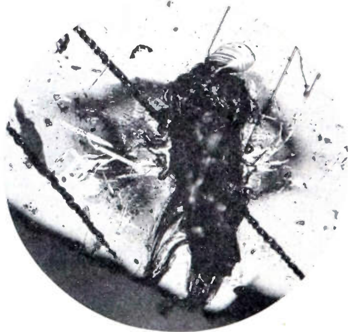
Fig. 4—Crater produced in germanium by heavy pulsing.
