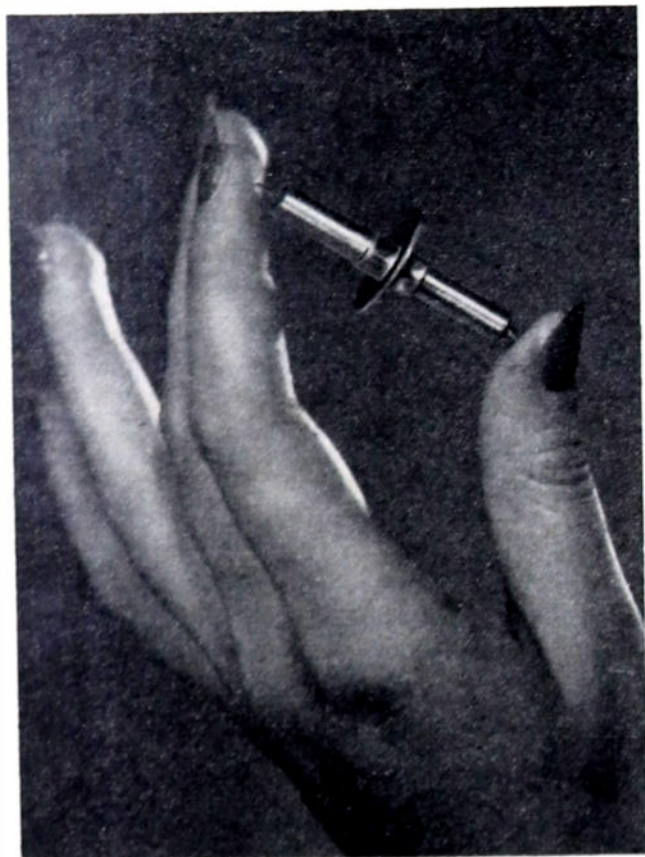
Fig. 4—A new "pencil triode," a medium- \mu type that is capable of producing peak output of more than 1,000 watts in plate-pulsed service at frequencies up to 3,300 mc (RCA).
