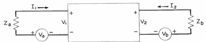
Fig. 2—Diagram of linear four-pole with terminations.
