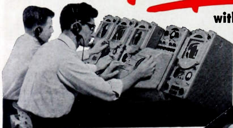
New GPL Video Switcher set up with two camera control units, a film chain control unit, and master monitor. This studio quality, field size switcher accommodates 5 cameras, 2 incoming lines.
