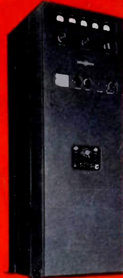
Collins 16F high frequency Autotune transmitter. The power output is 300 watts voice or MCW, 300 watts CW.
