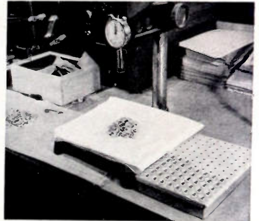
Inspection and Gaging . . . equipment for checking "E" dimensions of Disc Cathodes.
