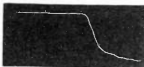
Amplified 20 \times 10^{-9} rise time pulse
