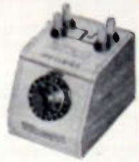
MODELS A, B, & C HELIPOTS A—10 turns, 46" coil, 1-13/16" dia., 5 watts—resistances from 10 to 300,000 ohms. B—15 turns, 140" coil, 3-5/16" dia., 10 watts—resistances from 50 to 500,000 ohms. C—3 turns, 13-1/2" coil, 1-13/16" dia., 3 watts—resistances from 5 to 50,000 ohms.
