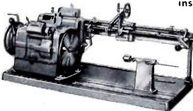
**MODEL AWO-A SMALL ARMATURE WINDER**—Fully automatic for mass production of small two-pole armatures with straight or skewed slots. Wire is guided by adjustable guide blade. Wire sizes (without insulation) from 23 to 44 SWG. Winding speed 700 RPM.
