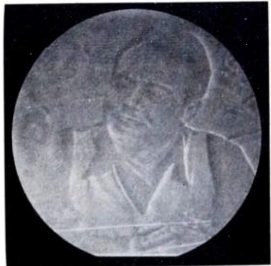
Fig. 6—Velocity reproduction of scene from broadcast received from WSB-TV. This photograph shows some evidence of signal integration performed by the uncompensated sweep amplifier.
