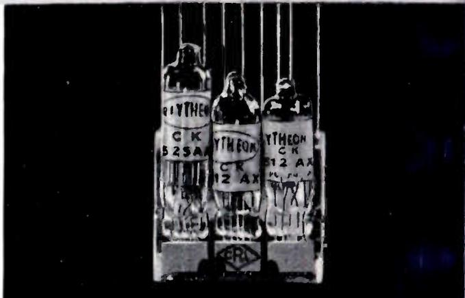
Ampec is a full 3-stage, 3-tube speech amplifier. Gives you truly highly efficient reliable performance. Size:  $1\frac{1}{4}$ " x  $1\frac{1}{8}$ " x .340" over tube sockets! Widely used in hearing aids, mike preamps and other amplifier applications where small size and outstanding performance counts. Bulletin No. 973 in coupon below.
