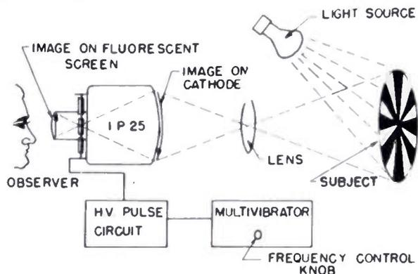
Fig. 6—Block diagram of stroboscopic application.
