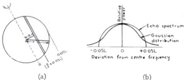
Fig. 7—(a) Effect of the moon's libration ( $L^\circ$ /day). The strip shown produces a frequency displaced  $[(a/r) \times 0.05L]$  cps from the center frequency. (b) Frequency spectrum of echo, assuming uniform brightness across the moon's disk, together with the closest-fitting Gaussian distribution.
