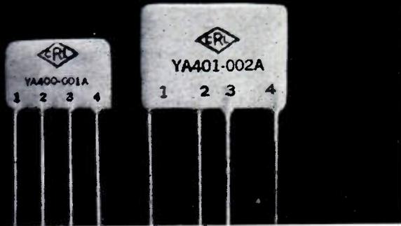
Centralab Triode Couplates save space and weight. They actually replace 5 components normally used in audio circuits. Triode Couplates are complete assemblies of 3 capacitors and 2 resistors bonded to a dielectric ceramic plate. Available in a variety of resistor and capacitor values. Bulletin No. 42-6 in coupon below.
