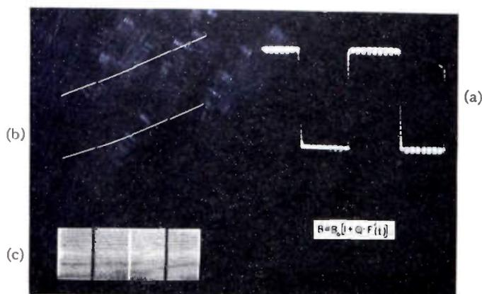
Fig. 2—Velocity reproduction of square-wave signal. (a) Signal superimposed on horizontal sweep voltage, (b) portion of expanded raster, and (c) resulting image.
