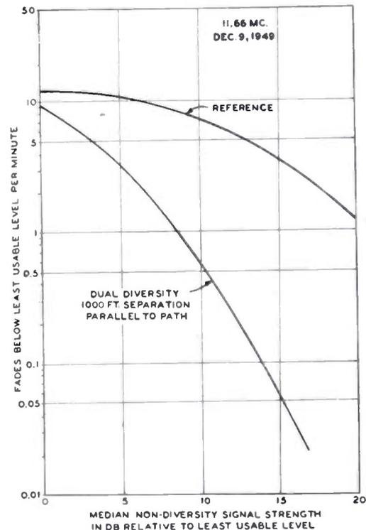
Fig. 3—Typical fading characteristics for a single day depicting the number of fades per minute below the respective levels.
