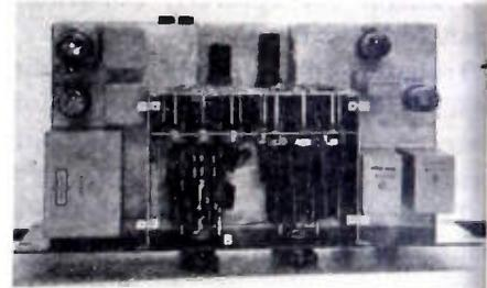
Fig. 3—Top view of decade oscillator showing tuning elements.
