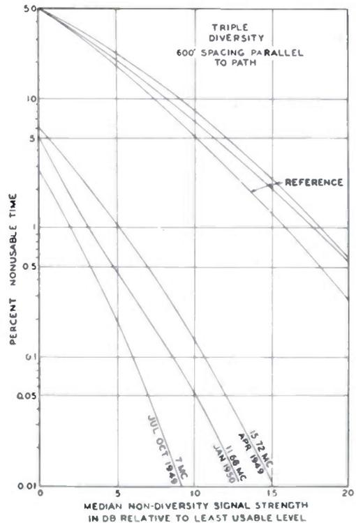
Fig. 12—Performance of triple-spaced-antenna diversity system for various seasons and frequencies.
