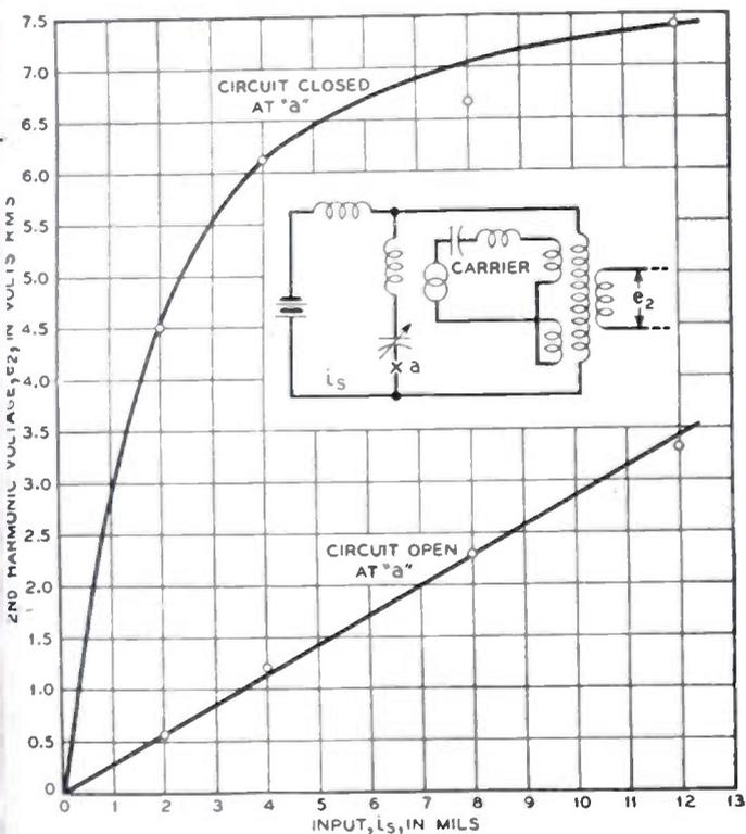
Fig. 13—Effect of a resonance in the input circuit.
