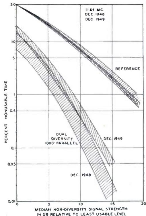
Fig. 7—Difference in performance of dual-spaced-antenna diversity system over interval of one year.
