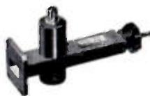
For measurement of power between frequencies 2.6 to 18.0 kmc in conjunction with -hp- 430A Power Meter and Sperry 821 barretter. Also may be employed to measure relative level, or detect rf energy using a Type 1N21 crystal. Each mount is semi-tuned by means of a movable short. Additional tuning may be provided if desired by means of -hp- 870A Slide Screw Tuner or -hp- 880A E-H Tuner. Sizes: 3" x 1½" (for use with barretter only), 2" x 1", 1½" x ¾", 1¼" x ⅝", 1" x ½", .702" x .391".
