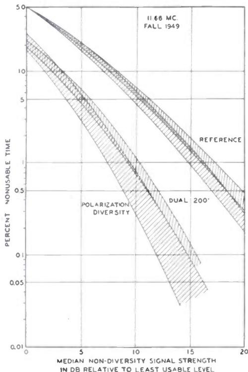
Fig. 15—Performance of inverted-L polarization diversity system showing typical variability in data. Performance of dual-spaced-antenna diversity is shown for comparison.
