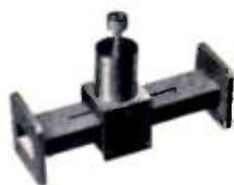
For flattening waveguide systems. Consists of slotted waveguide section and adjustable probe on sliding carriage. Varying position and penetration of probe sets up VSWR which can be adjusted to cancel existing VSWR in system. VSWR
