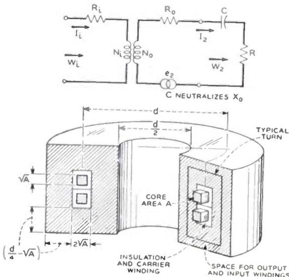
Fig. 10—(a) Simplified magnetic amplifier circuit. (b) Cutaway drawings showing physical arrangement of cores and windings.
