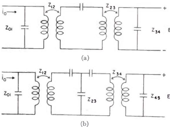
Fig. 1—Typical circuit configurations. (a) Triple-tuned circuit (b) Quadruple-tuned circuit.
