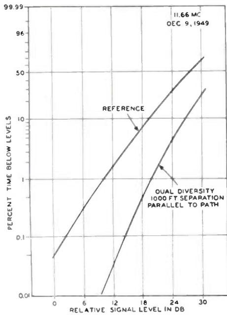
Fig. 1—Typical results plotted on Rayleigh co-ordinates. Data are for a single day.
