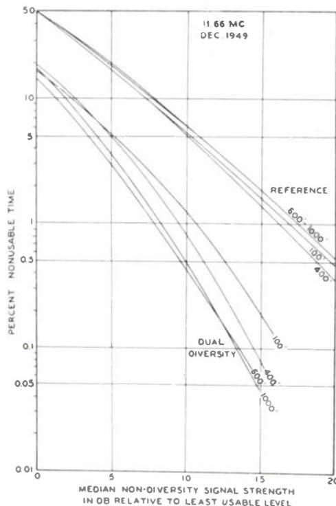
Fig. 8—Effect of antenna spacing on performance of dual-spaced-antenna diversity system.
