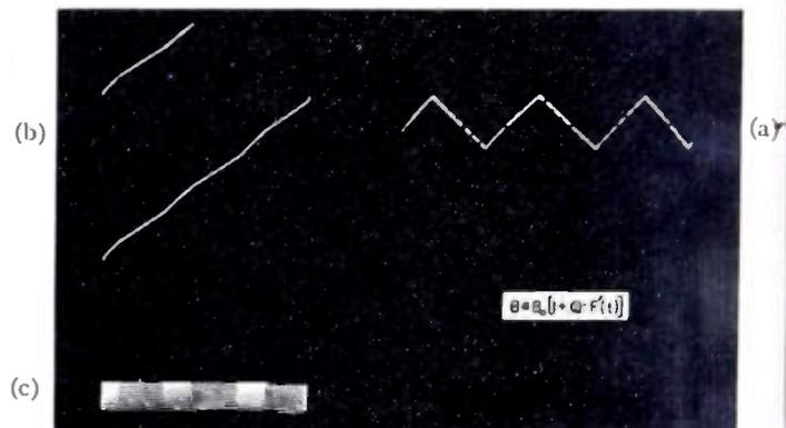
Fig. 3—Velocity reproduction of pyramid signal. (a) Signal superimposed on horizontal sweep voltage, (b) portion of expanded raster, and (c) resulting image.
