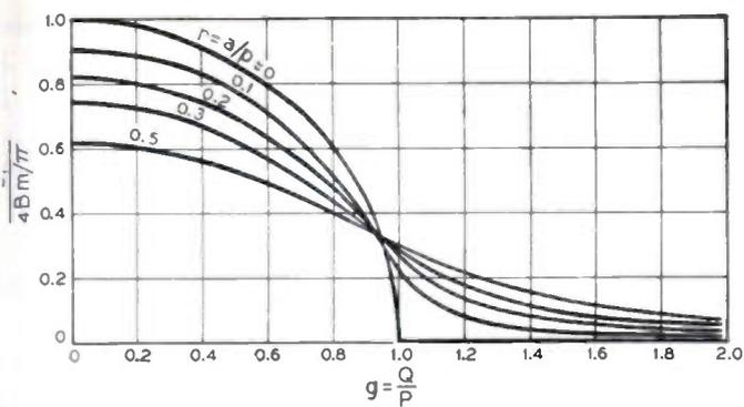
Fig. 7—Fundamental component of flux density as a function of bias.
