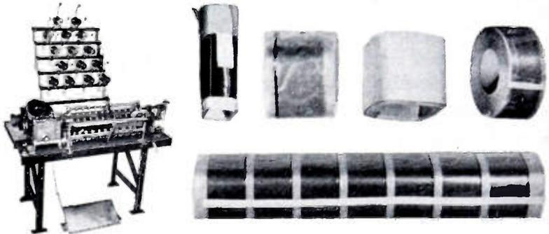
Transformer winder Model 37S multiple winds power, audio, automotive, fluorescent ballast and similar types of coils. Winds wire from No. 18 B&S to 46 B&S up to 9" O.D. Maximum economy is possible by using mandrels up to 30" long. Thirty or more coils may be wound at one time. All turns are accurately registered by Model 50 or 51 6" full vision clock face Dial Counter. Set-ups can be changed in less than 5 minutes. A gear chart is furnished to quickly determine wire spacing.
