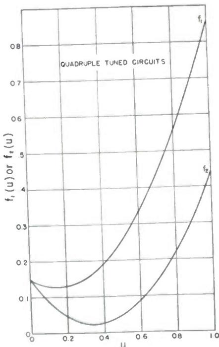
Fig. 4—Design functions for quadruple-tuned circuits.
