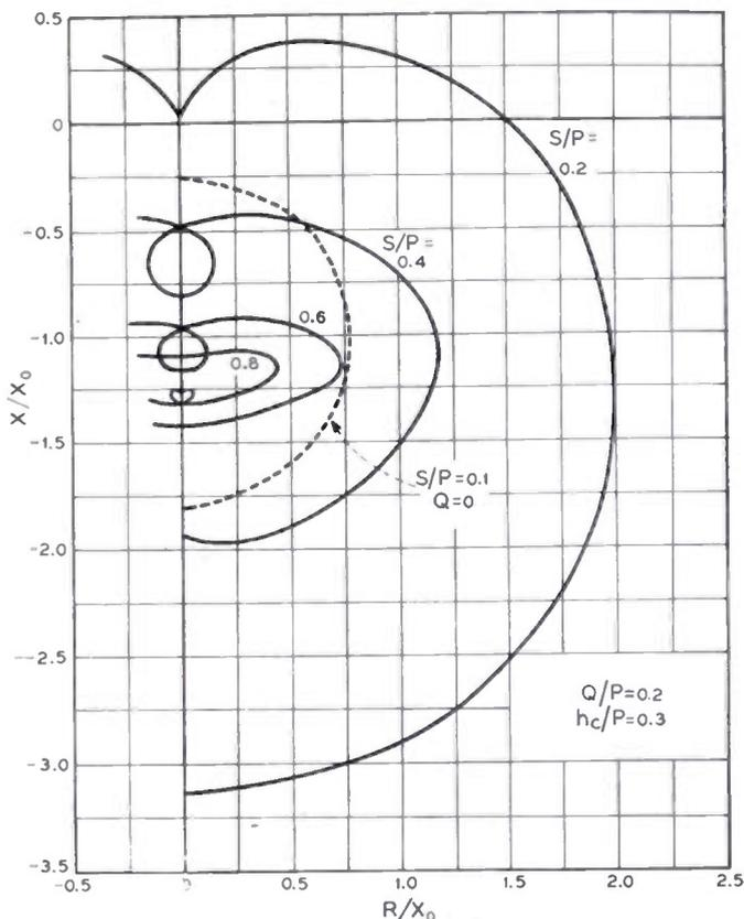
Fig. 8—Second-harmonic current computed as a function of external impedance.
