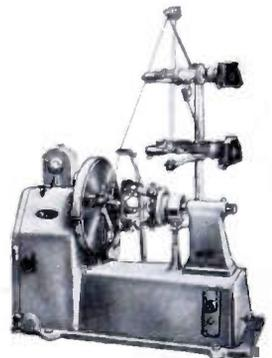
**MODEL OOFA-PEM MULTIPLE FINE-WIRE WINDER** with fully automatic paper interleaving device, for flanged or flangless coils. Winds up to 6 coils at a time with individual paper interleaving. **MODEL OOFA-PEB** winds up to 10 flangless coils with common paper interleaving. Wire sizes from 24 to 44 AWG. Winding speeds from 360 to 3000 RPM.
