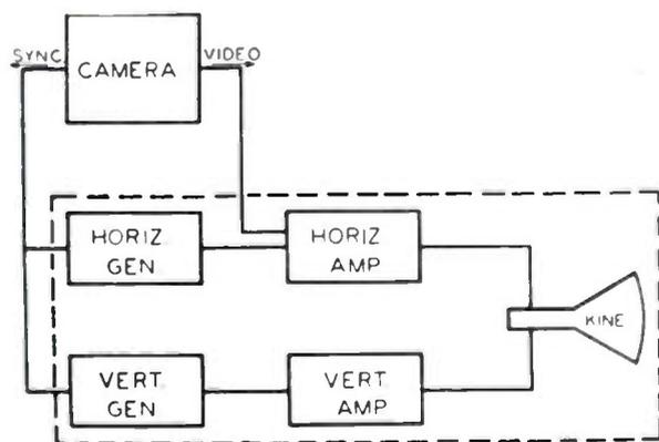
Fig. 1—Experimental velocity-modulation reproduction system.
