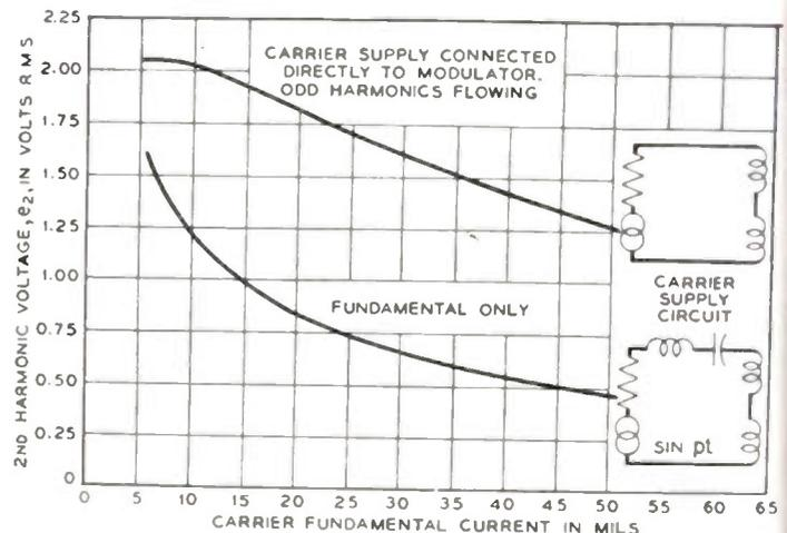
Fig. 12—Effects of supplying carrier current in two different ways.
