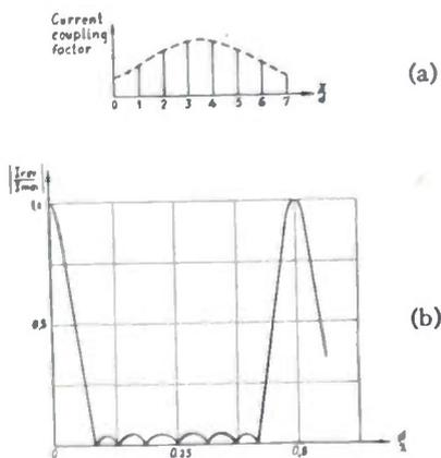
Fig. 1—Diagrams of a directional coupler which optimizes the relationship between pass-bandwidth and the allowed  $I_{rev}/I_{max}$  level in the pass band.
