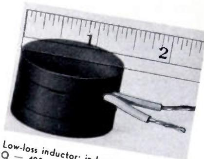
Low-loss inductor: inductance = 1 henry;  $Q = 400$  at 30 kc. Extremely low-loss inductors and high-fidelity transformers are obtainable over a wide range of values and frequencies, using similar structures in various physical sizes.
