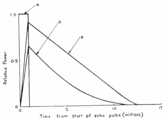
Fig. 6—Shape of echo pulse for a 1-millisecond incident pulse. (a) Smooth moon. (b) Rough moon, Lambert scattering. (c) Rough moon, Lommel-Seeliger scattering. The unit of power is that for a smooth moon and long pulses.
