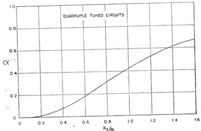
Fig. 5—Flatness parameter for quadruple-tuned circuits.
