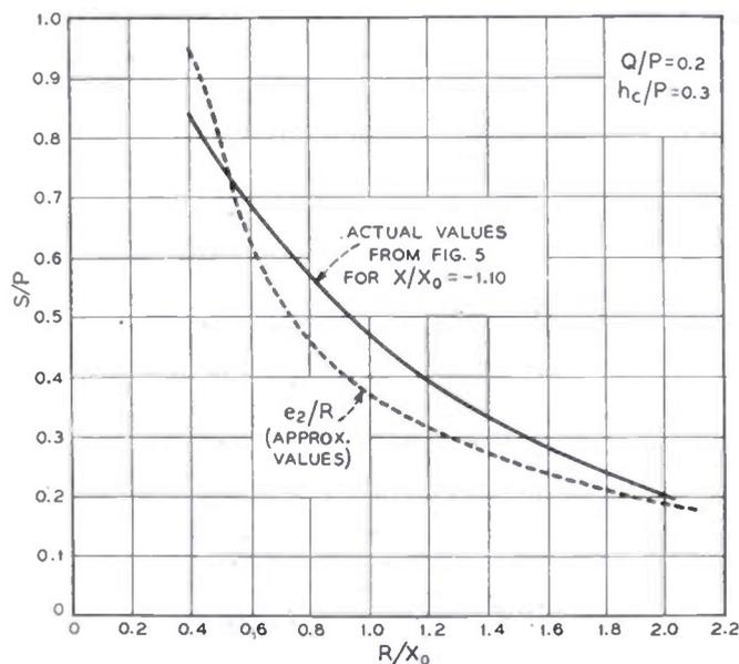
Fig. 9—Second-harmonic current as a function of external resistance for a fixed value of reactance.
