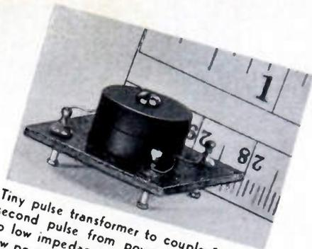
Tiny pulse transformer to couple 2 microsecond pulse from power amplifier tube to low impedance load. We can produce low power pulse transformers to reproduce pulses of widths ranging from a fraction of a microsecond to several milliseconds.
