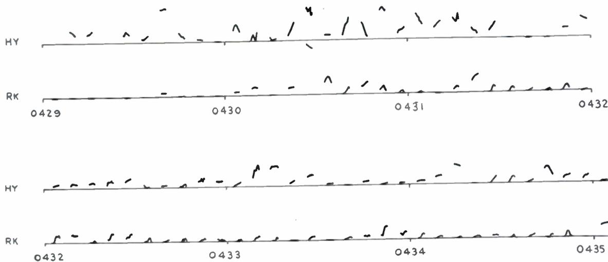
Fig. 4—Simultaneous records of echo strength at Hornsby (HY) and Rockbank (RK), 0429–0435 E.A.S.T., October 29, 1948. The scales are linear in voltage, the Hornsby record being drawn to twice the scale of the Rockbank one.
