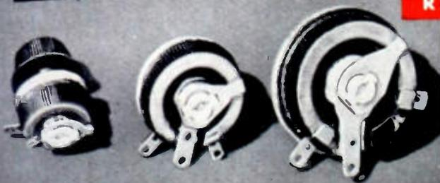
The Ohmite series of standard, close control rheostats is the most extensive available—so it is easy to select a size to fit your application. There are ten sizes, ranging from 25 to 1000 watts, with many standard resistance values in each size. All models have the Ohmite all-ceramic construction, with winding permanently locked in vitreous enamel, and smoothly gliding metal-graphite brush.
