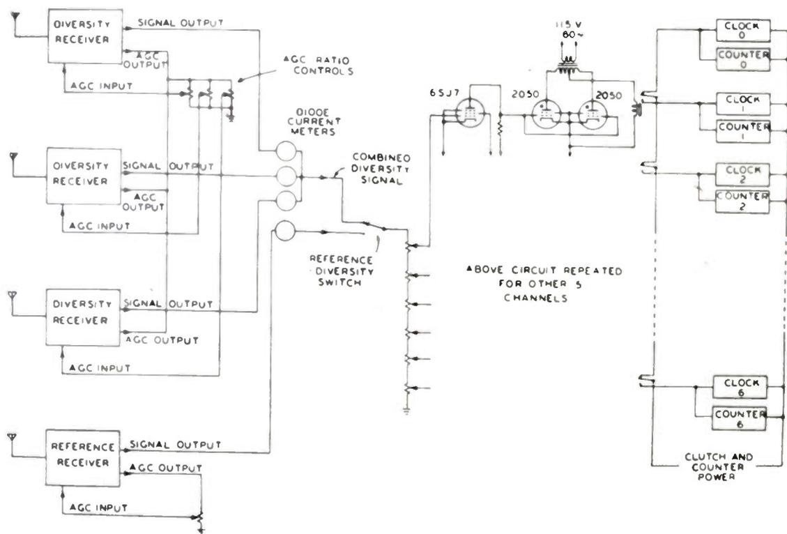
Fig. 3—A simplified diagram of the recording instrument.
