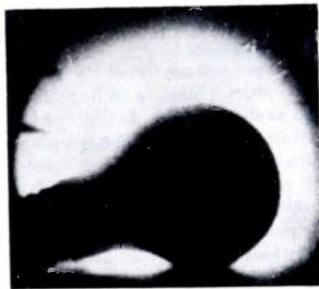
Fig. 4—Two-microsecond-exposure shadowgraph of light bulb.
