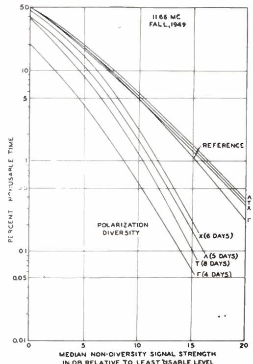
Fig. 18—Comparative performance of various polarization diversity systems. The systems differ only in the physical arrangement of antennas.
