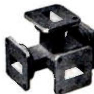
Four-arm, rectangular hybrid tee. Composed of series and shunt tee constructed at same point in waveguide. Possess many properties of bridge circuit. Used for rapid determination of VSWR; as impedance transformer; as a bridge, etc. Sizes: 3" x 1½", 2" x 1", 1½" x ¾", 1¼" x ⅝", 1" x ½", .702" x .391".
