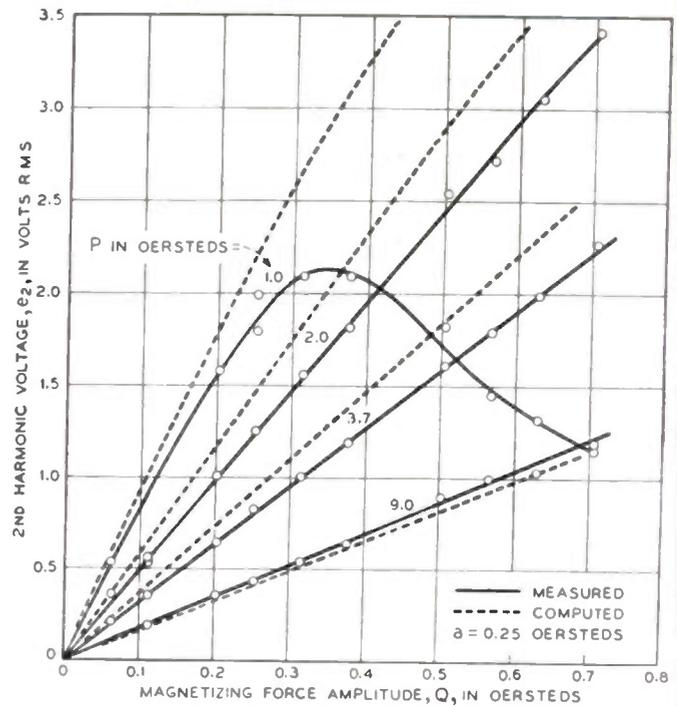
Fig. 5—Measured and computed values of second harmonic voltage.
