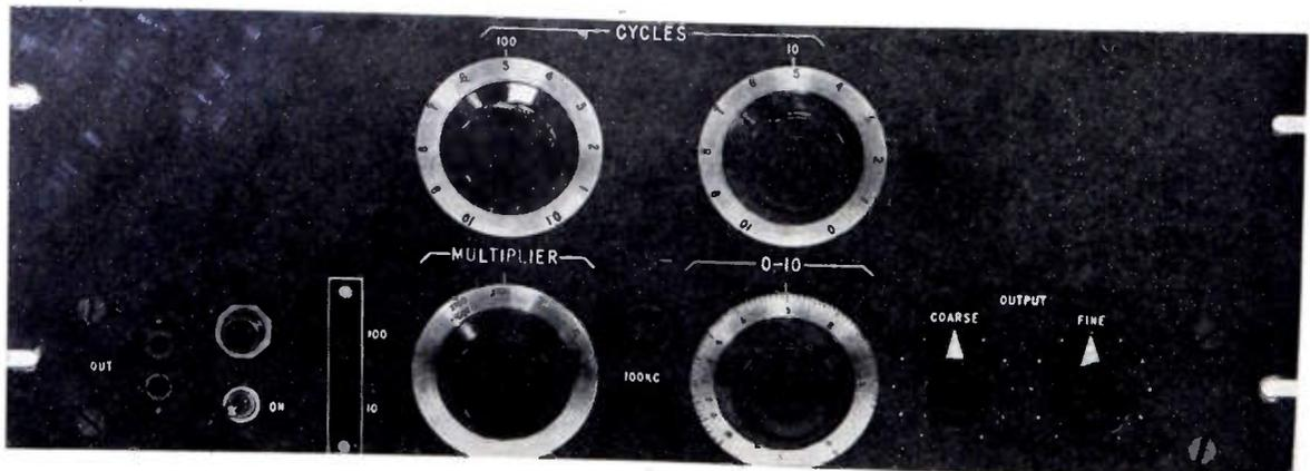
Fig. 2—Front view of decade oscillator showing dials.
