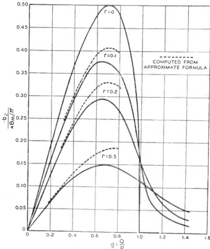
Fig. 4—Second-harmonic flux-density component as a function of bias.
