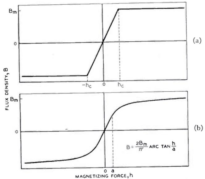
Fig. 3—*B-H* characteristics.
