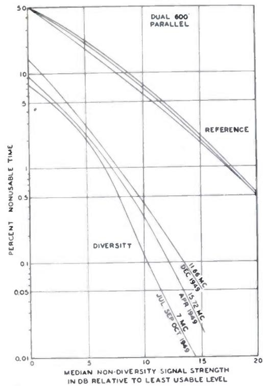
Fig. 6—Performance of dual-spaced-antenna diversity system for various seasons and frequencies.
