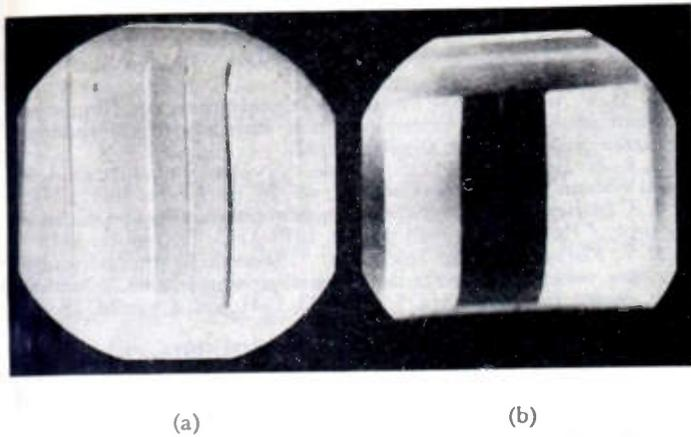
Fig. 4—Vertical black bar with narrow test wedge reproduced by (a) velocity modulation and by (b) conventional methods.
