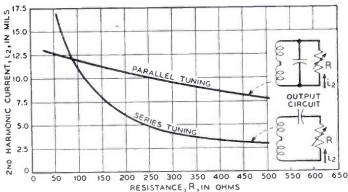
Fig. 14—Effects of two different ways of tuning the output circuit.
