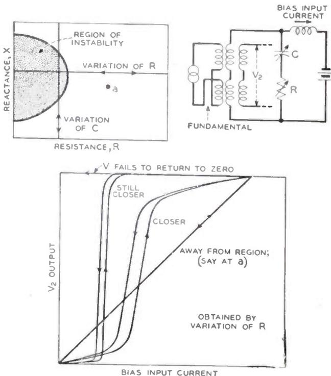
Fig. 11—Diagrams showing effect of regeneration because of second harmonic current.
