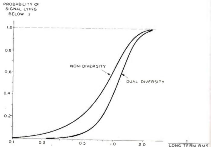
Fig. 1—Curves showing the probability that a nondiversity and a dual-diversity signal amplitude will at any instant be less than a designated amplitude. Uncorrelated Rayleigh distributed fading on the two diversity channels is assumed.
