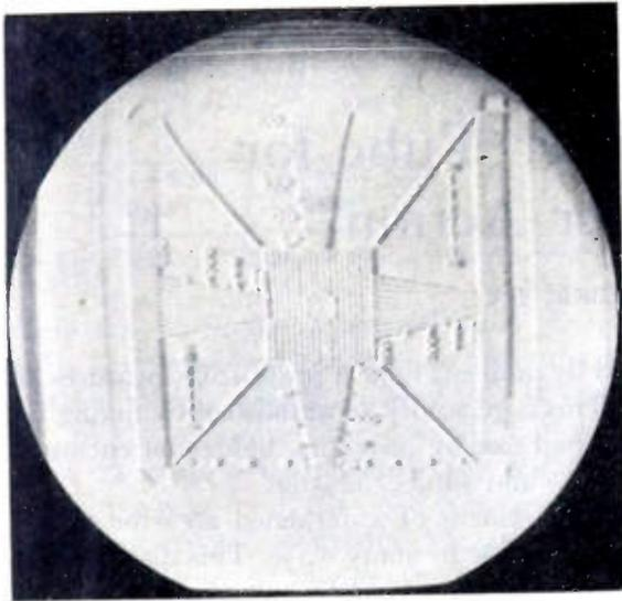
Fig. 5—Standard test pattern reproduced by velocity modulation.
