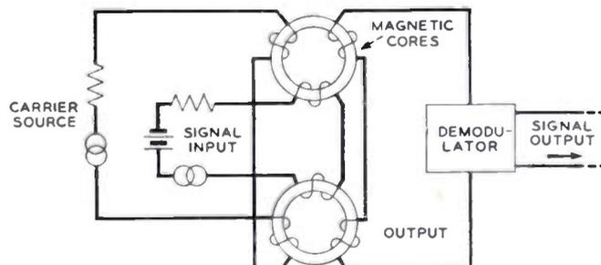
Fig. 2—Arrangement of cores and windings for one type of magnetic amplifier.
