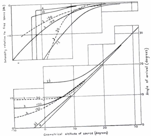
Fig. 10—One-way transmission through *F*-region (ray theory). (a) Intensity against geometrical altitude. (b) Angle of arrival against geometrical altitude. The full-line curves are for  $f/f^{\circ}_{F_2} = 2\frac{1}{2}, 3, 3\frac{1}{2}, 4$ , height = 250 km, semithickness = 100 km and the dashed-line curves for  $f/f^{\circ}_{F_2} = 3$ , height = 250 km, semithickness = 50, 150 km.
