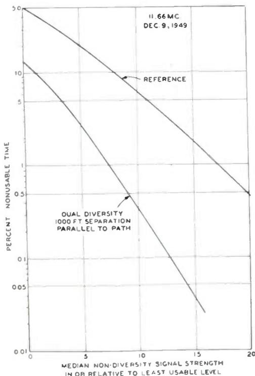
Fig. 2—Typical fading characteristics for a single day relative to median value of signal strength received on the reference system.
