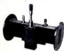
For use between 2,600 and 3,950 mc to create known attenuations or isolate sources and loads. Each instrument accurately calibrated at 3,000 mc. Max. VSWR 1.15. Sizes: 3" x 1½". (Other sizes to be announced.)
