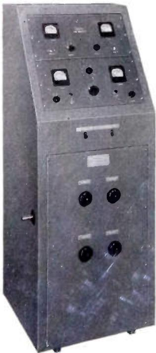
This instrument is a simplified, portable Mass Spectrometer, specifically designed to be extremely sensitive to Helium.
