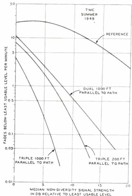
Fig. 14—Performance of triple-spaced-antenna diversity system with respect to fades per minute below respective levels.
