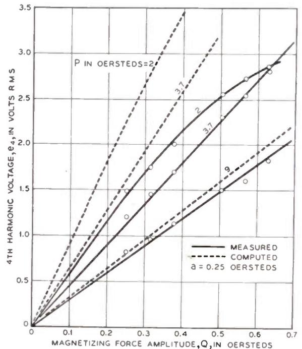
Fig. 6—Measured and computed values of fourth harmonic voltage.
