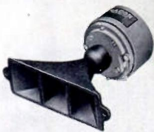
Model CHU-5 provides uniform response to 12,000 cps with usable output to beyond 15,000 cps. When used with a 2- to 15-inch cone speaker and proper network, it handles 25 to 30 watts of program material. Its impedance is 15 ohms.
