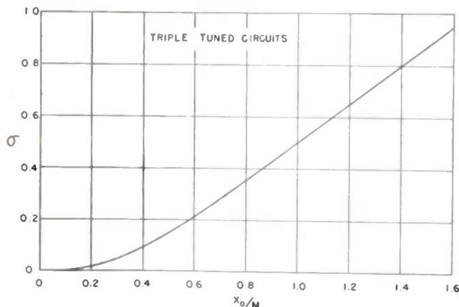
Fig. 3—Flatness parameter for triple-tuned circuits.
