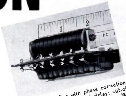
Lumped delay line with phase correction: 1750 ohm; 20 microsecond delay; cut-off frequency of 200 kc; 1/2 db power loss. We are prepared to make delay lines covering the audio and radio frequency spectrums.
