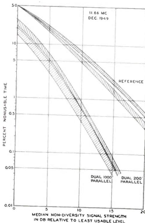
Fig. 4—Performance of dual-spaced-antenna diversity system showing typical variability in data.
