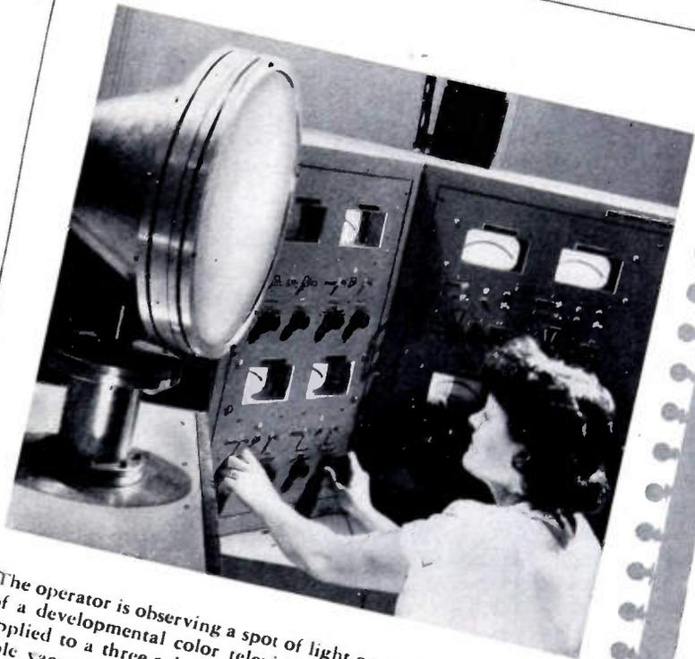
The operator is observing a spot of light on the phosphor screen of a developmental color television tube. By varying voltages applied to a three-color electron gun inserted in the demountable vacuum system, she can obtain data useful in improving both phosphors and gun designs for color television tubes.
