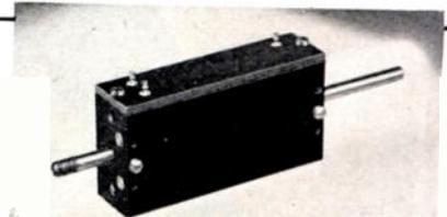
**Type RV3\* Bakelite Base Precision Potentiometers** . . . available in models for either linear or non-linear functions. Stock resistance values ranging from 100  $\Omega$  to 200,000  $\Omega$  and power ratings of 8 and 12 watts. 360° mechanical rotation or limited by stops as desired. Potentiometers of this type available to widely varying accuracy requirements (linearity to  $\pm 0.25\%$ ) — see TIC Bulletin RV3-250. Special models available for high humidity applications.
