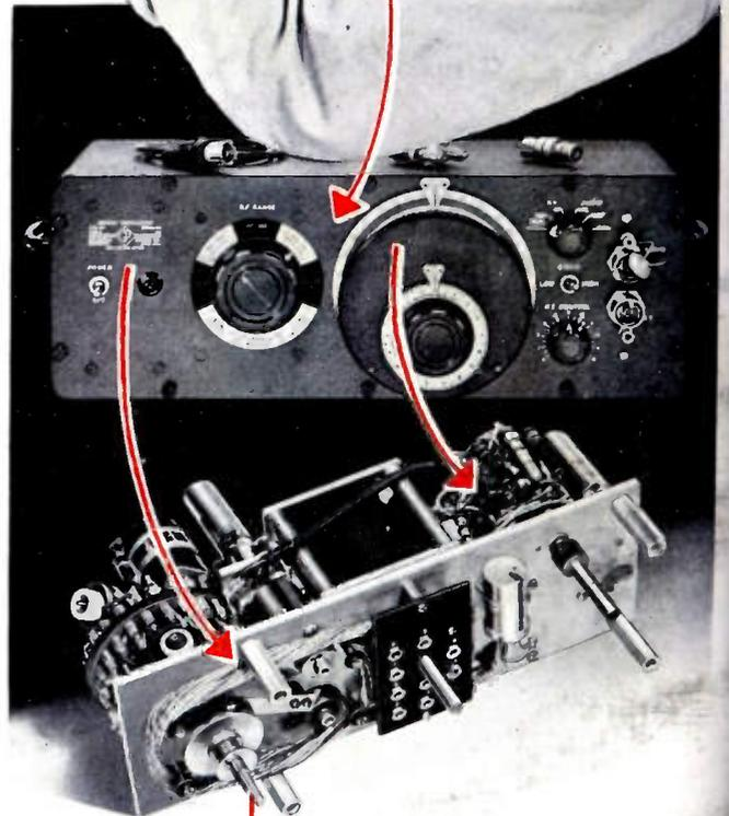
Excellent mechanical construction throughout. Oscillator assembly plugs into deep brass box; double cover completes shielding. Note servicing cable permitting instrument to be tested on bench.
