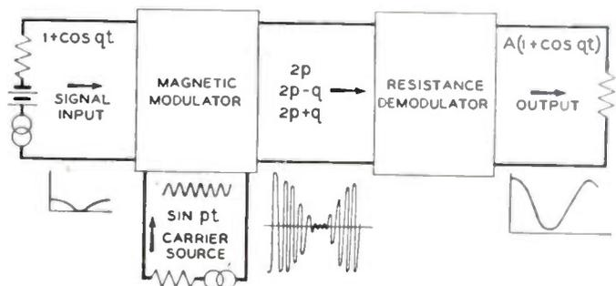
Fig. 1—A magnetic amplifier pictured as a carrier system.
