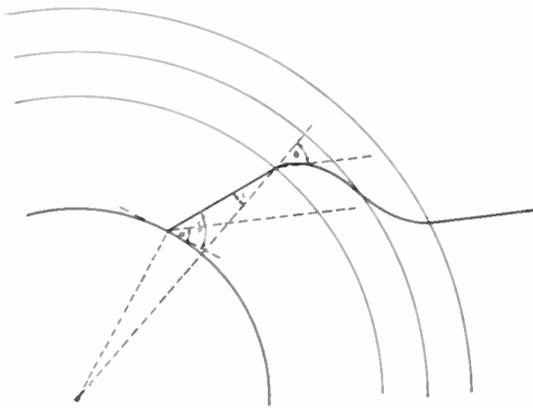
Fig. 9—Trajectory of ray through ionosphere.
