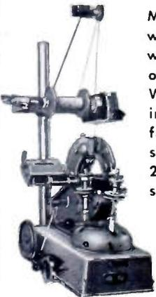
**MODEL RW TOROIDAL WINDER** with Coil Supports—automatically winds toroidal coils around 360° or sector coils up to 270°. Winds in either direction. Made in three sizes for single wire from 18 to 38 AWG, double or stranded wires from 2 x 18 to 2 x 26 AWG. Maximum winding speed 200 RPM.
