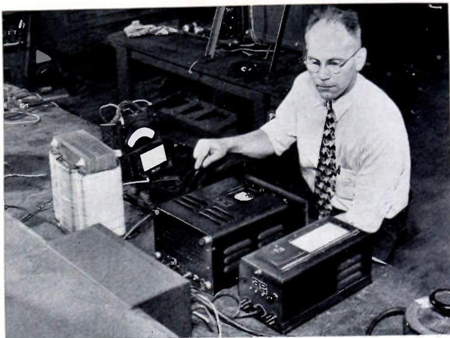
WHILE THE ELECTRONS FLOW, this Brush D.C. Amplifier and Oscillograph measures and records the time constants of a reactor, eliminating hours formerly required for plotting. Write for Bulletins 460 and 540.
