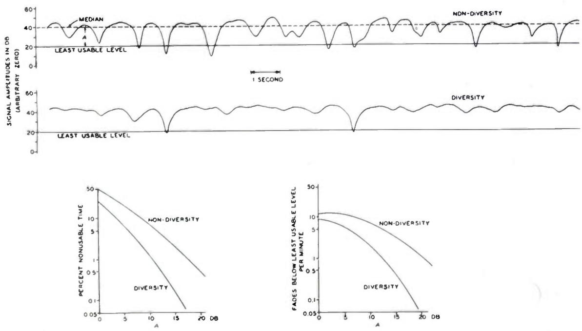
Fig. 2—An example showing the dependance of nonusable time and fades below least usable level upon the strength of the received signal relative to the least usable level.
