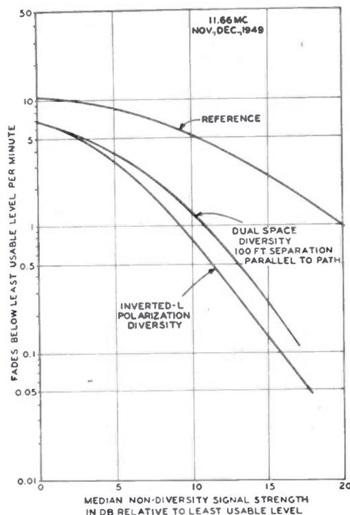
Fig. 16—Performance of inverted-L polarization diversity system with respect to fades per minute below respective levels.
