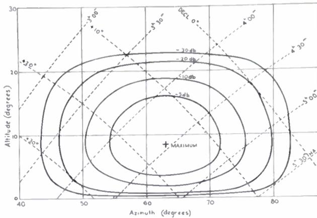
Fig. 1—Composite aerial diagram of the Shepparton transmitter and Hornsby receiver, plotted in terms of azimuth and altitude at Shepparton. Contours of declination and hour angle are also shown.
