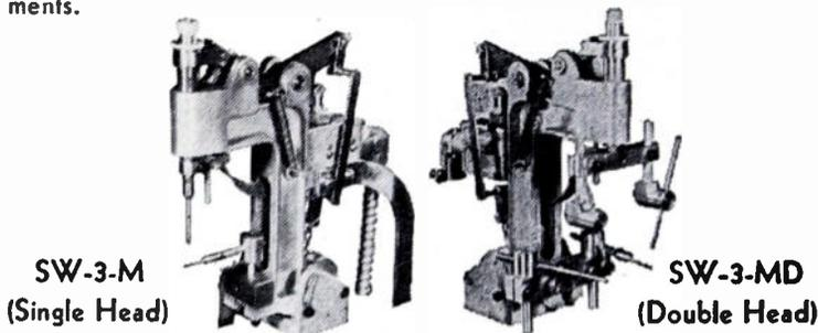
Both units are 3½" wide, 10½" high, 8" deep. The heads can be tilted backwards 30° from normal upright position. Power supply available for these welders in kilowatt ratings of ¼, ½, ¾, 1, and 2 KVA stepless power control.
