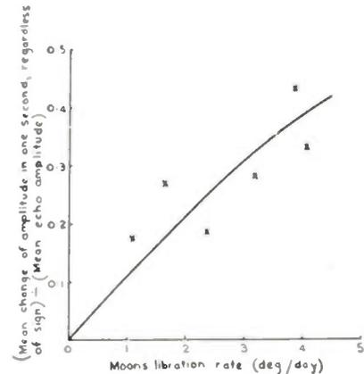
Fig. 8—Relation between speed of rapid fading and libration rate. The full line is the theoretical curve, while the crosses indicate experimental points for six days.
