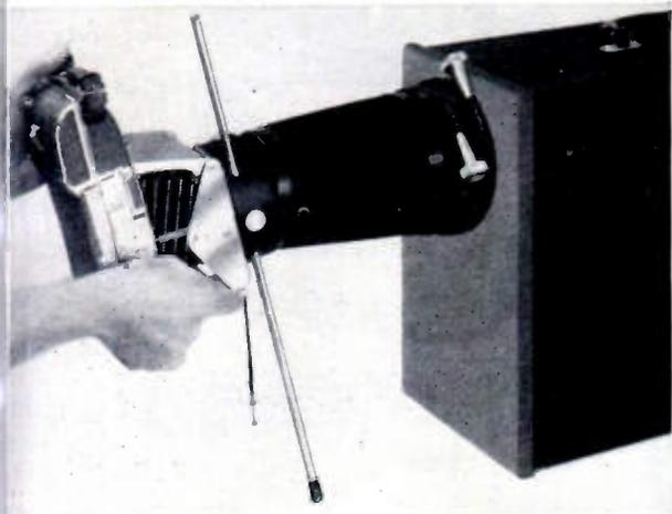
**Set up the camera.** The Fairchild-Polaroid camera consists of three units: adapter ring, hood, and camera body. To set it up, you place the handy adapter ring over the oscilloscope bezel, slip the hood into the ring, then snap the camera into the bayonet lock on the hood. That supporting rod is a safety feature that protects both camera and oscilloscope.
