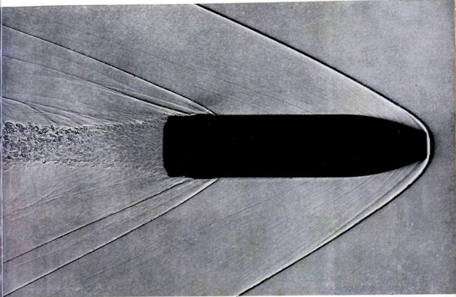
Velocity of projectile: Approx. 2800' per second. Duration of spark light:  $12 \times 10^{-7}$  second.
