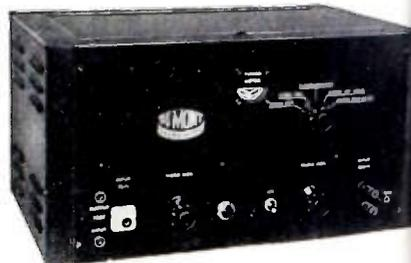
The Dumitter is a compact, completely portable unit. It takes the composite video signal from any standard TV camera chain, and feeds it via a single coaxial cable to the antenna terminals. A carrier signal of the frequency of either Channel 2 or 3 (optional on the Dumitter controls) is used. Up to 125 receivers can be driven simultaneously, with transmission of over several thousand feet.
