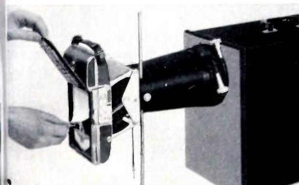
**Remove the finished print.** A minute after you've pulled the tab, the finished print is ready for evaluation. Just open the camera back and there it is. An easy job, but you have a photographically accurate record of the trace in less time than you could sketch it from memory.
