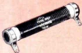
Type MV High Voltage Resistors utilize IRC's famous filament resistance coating in helical turns on a ceramic tube to provide a conducting path of long, effective length. Result: Exceptional stability even in very high resistance values. Catalog Bulletin G-1.
