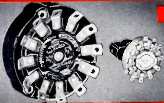
Ohmite tap switches are supplied in five standard models, rated at 10, 15, 25, 50, and 100 amperes, a.c. They combine high current capacity and a large number of taps with unusual compactness. Their sturdy, one-piece ceramic bodies provide permanent non-arcing insulation. Their heavy silver-to-silver contacts have a self-cleaning action and provide continuous, dependable contact with low resistance. Ohmite tap switches are supplied in enclosed or open, shorting or non-shorting types.
