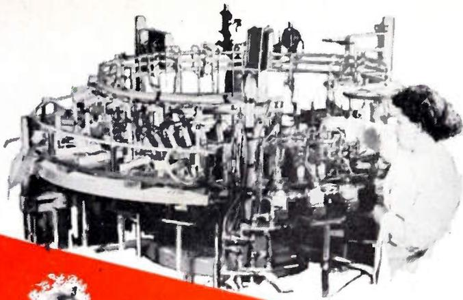
This 32-head exhaust unit, shown at the left, is one of the many specially designed machines used by Haydu Brothers to insure the high vacuum of all small tubes at high production rates. Stage-tests at intervals throughout production guarantee complete *quality* control!
