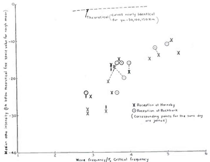
Fig. 11—Relation between median echo intensity and  $f^\circ F_2$ .
