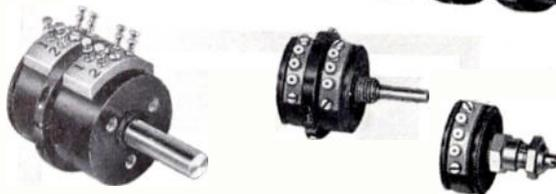
**RVP3\* High Precision machined aluminum base Potentiometers** . . . available in models for either linear or non-linear functions with standard resistance values up to 200,000  $\Omega$ . Linearity to  $\pm 0.1\%$ . Eleven gang assembly shown — example of TIC's potentiometers multi-ganged with TIC's adjustable clamp ring. Can be supplied to meet various mounting requirements — single hole, 3 tapped hole mounting or servo mounting as desired.
