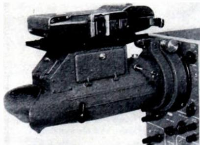
The camera employs the Polaroid-Land process for delivering a finished print at the termination of each completed exposure or set of exposures. By means of a sliding mount, the camera may be positioned so that several traces can be recorded on a single print, for side-by-side comparisons. There is also a built-in detent which divides a single print into one, two, or three separate exposure areas.
