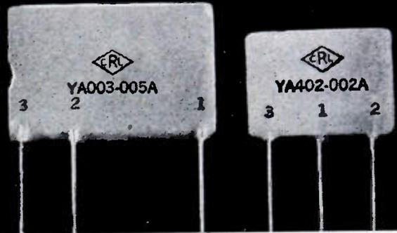
Centralab Vertical Integrators give you big savings in assembly costs, particularly in TV vertical integrator networks. One type consists of 4 resistors and 4 capacitors brought out to 3 leads... reducing the formerly required 16 soldered connection to only 3! There's a big saving in the number of parts handled, too! Bulletin No. 42-22.
