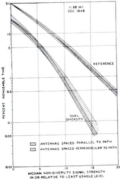
Fig. 10—Effect of orientation of antenna array with respect to signal path on performance of dual-spaced-antenna diversity system.
