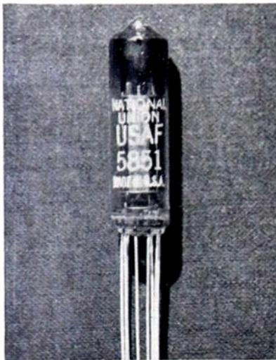
Designed for use in military and other applications where the tube is subjected to excessive shock and vibration, this tube is suitable for frequency doubler operation up to 400 Mc producing 120 milliwatts. The 5851 filament requires only 55 ma current at 2½ volts; it also may be operated at 1½ volts at 110 ma.
