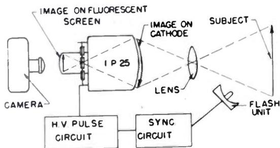
Fig. 2—Block diagram of photographic system.
