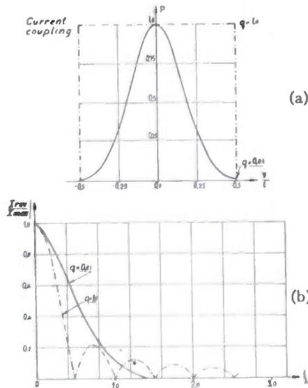
Fig. 2—Diagrams of directional couplers consisting of continuous slots.
