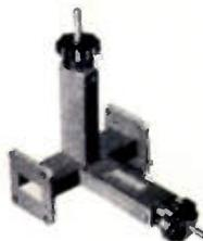
Matching section for tuning high power systems or for tuning systems where low leakage is essential. Consists of hybrid waveguide tee with moveable choke type shorts placed in shunt and series arms. Sizes:  $3'' \times 1\frac{1}{2}''$ ,  $2'' \times 1''$ ,  $1\frac{1}{2}'' \times 3\frac{3}{4}''$ ,  $1\frac{1}{4}'' \times 5\frac{5}{8}''$ ,  $1'' \times 1\frac{1}{2}''$ ,  $.702'' \times .391''$ .
