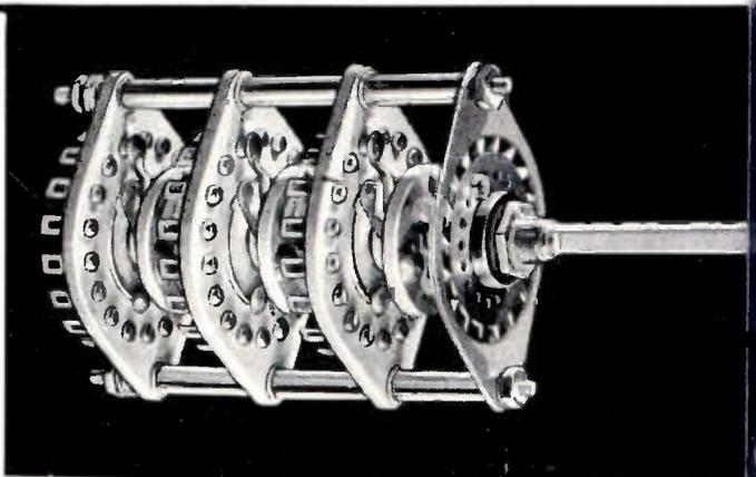
Medium Duty Power Switch for R.F. or  $7\frac{1}{2}$  amp. 110-115 V. application. 1, 2 or 3 poles . . . 18 contact sections . . . up to 20 sections per shaft. Contacts, collector rings coin silver mounted on Grade L5 Steatite. Cat. No. 722.
