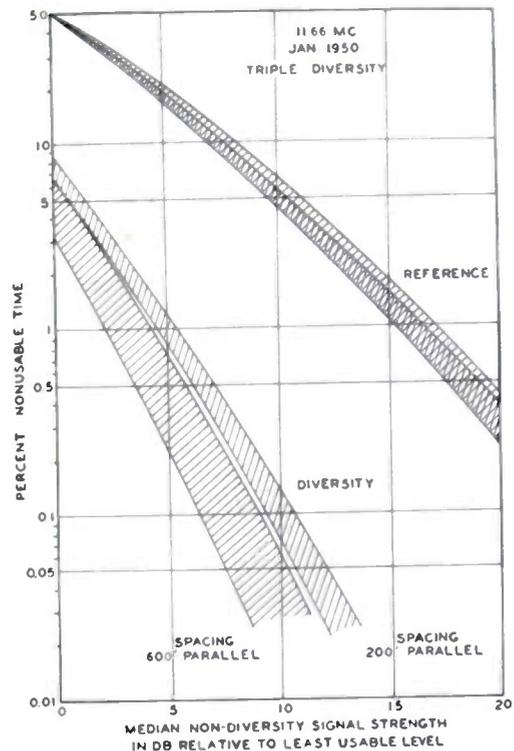
Fig. 11—Performance of triple-spaced-antenna diversity system showing typical variability in data.
