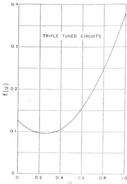
Fig. 2—Design function for triple-tuned circuits.
