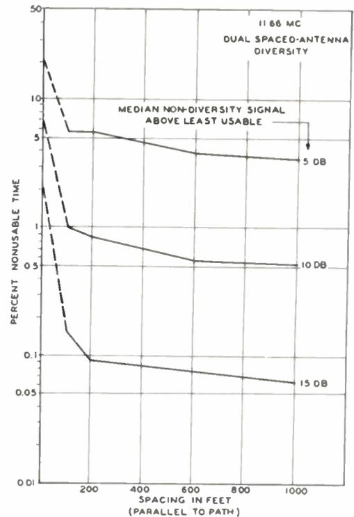
Fig. 9—Influence of spacing on performance of dual-spaced-antenna diversity system.
