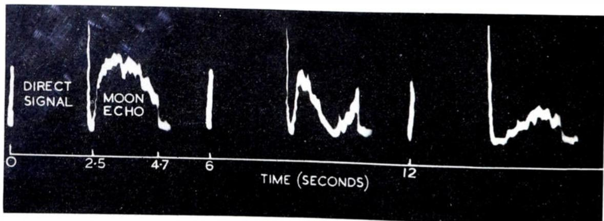
Fig. 3—Three successive echoes obtained with 2.2-second signals, illustrating the rapid fading. The small fluctuations are due to cosmic noise, passed through an intermediate-frequency bandwidth of 70 cps and video bandwidth of 6 cps.
