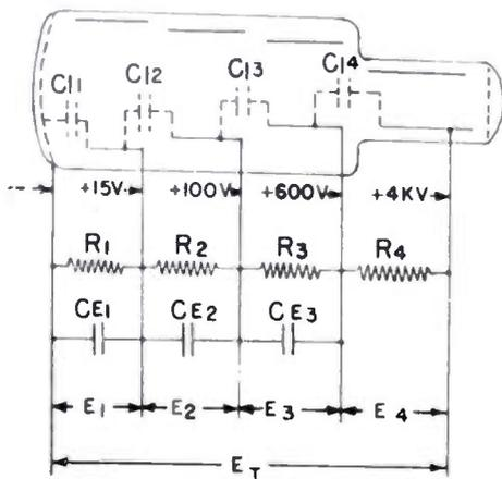
Fig. 7—Voltage divider circuit.
