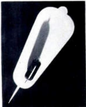
colloidal graphite dispersion as a coating on the outside of their CK1026 radiation counter tubes.
