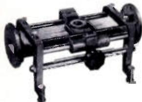
Slotted sections are one of the most important measuring instruments in waveguide engineering. They are essential to the measurement of impedance, reflection and other transmission characteristics.
