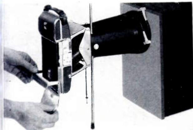
**Pull the tab to finish exposed print.** After a snap of the shutter, the exposure is made and you're ready to finish the print. If you want two exposures, it's easy to move the camera body down and make a second exposure. To finish the print, you merely pull tab at back of camera.
