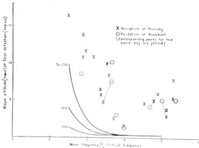
Fig. 12—Relation between altitude at first detection and  $f^{\circ}F_2$  for the lower of the two rays. The full lines are theoretical curves, derived from the ray-theory treatment of Subsection IV, E, for a symmetrical parabolic  $F_2$  region of height 250 km and semithickness 50, 100, 150 km, with account being taken of the aerial diagram.
