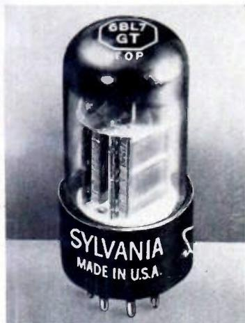
6BL7GT, also permits simplification and better performance when applied to TV circuits requiring two tubes for vertical deflection.
