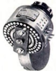
The 730 has zero insertion loss, a constant input and output impedance, and is suited for use where space is of importance. It is available in steps of 0.5, 1, 1.5, or 2.0 db. It has a flat frequency characteristic to 30 kc. On special order, the frequency range can be extended to 200 mc.
