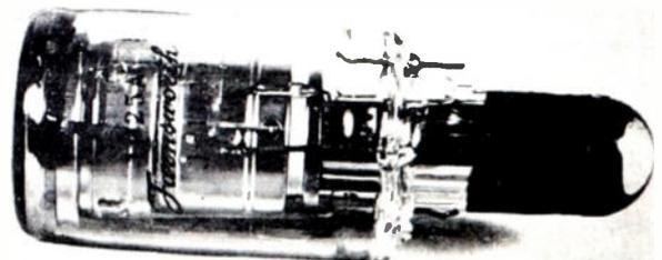
Fig. 1—Image converter tube.
