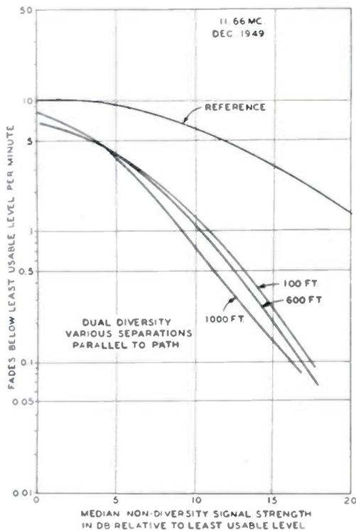
Fig. 5—Performance of dual-spaced-antenna diversity system with respect to fades per minute below respective levels.
