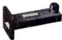
For transition between waveguide and coaxial systems. Each adaptor covers the full waveguide range with a VSWR not exceeding 1.5. -hp- 280A with flexible cable, 3" x 1½" only. -hp- 281A, with Type N Jacks, sizes 3" x 1½", 2" x 1", 1½" x ¾", 1¼" x ⅝", 1" x ½".
