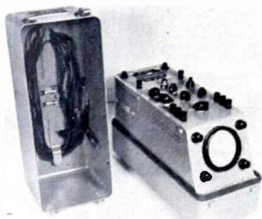
The wide-band and linearity features of the instrument have heretofore been found only in laboratory-type equipment. The sweep frequency range is from 3 to beyond 50,000-cps. Vertical amplifier response is flat within 3 db from dc to 2 Mc, while horizontal response is flat within 2 db from dc to 100 kc. Faithful reproduction of wave forms with 3 microsecond rise time and 100 kc square waves is an unusual feature.
