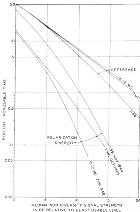
Fig. 17—Performance of T polarization diversity system for various seasons and frequencies.
