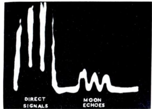
Fig. 2—Sample photographic record, illustrating the results obtained with the group of three short pulses.
