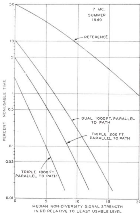
Fig. 13—Effect of antenna spacing on performance of triple-spaced-antenna diversity system. Performance of dual system is shown for comparison.
