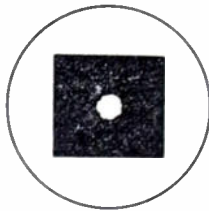
Fig. 70—Raster excitation for contrast measurement; raster area except center excited.
