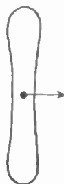
Fig. 12—Representation of the electric field intensity about a rapidly moving charge ( \kappa = 2 ).
