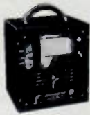
NO. 1020 DIRECT READING MEGOHMMETER Measures insulation resistances up to 2,000,000 megohms. 500 volts D.C. potential included in the instrument. Entirely self contained and A.C. operated.
