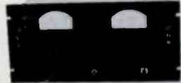
NO. 1210 NULL DETECTOR & VACUUM TUBE VOLTMETER Vacuum Tube Voltmeter: Sensitivity .1, 1, 10, 100 volts. Input impedance 50 megohms shunted by 20 mfd. Frequency range 20 cycles - 20,000 cycles. NULL DETECTOR: Gain 94 DB. Selective circuits for 40, 400, 1000 cycles. Frequency range 20-30,000 cycles.
