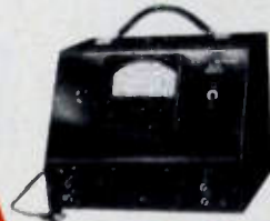
NO. 1060 VACUUM TUBE VOLTMETER For use at audio, super-sonic and radio frequencies. Frequency range from 10 cycles to 1.6 megacycles. Input impedance 50 megohms. Input capacity 15 MMF. Voltage range from .001 to 100 volts. Frequency range from 10 cycles to 2 megacycles.
