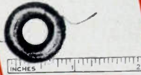
HI-Q MINIATURE TOROIDAL INDUCTORS Size 3/4" D. x 3/8" — weight 3/4 ounce. Type TI-5 Frequency range 1000 cycles - 15,000 cycles. Type TI-7 Frequency range 10,000 cycles - 100,000 cycles. Wound on molybdenum permalloy dust cores. Available in hermetically sealed cans, potted and cased or open units.
