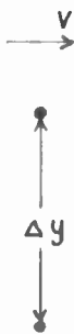
Fig. 11—Two electrons moving in a direction perpendicular to a line joining them.
