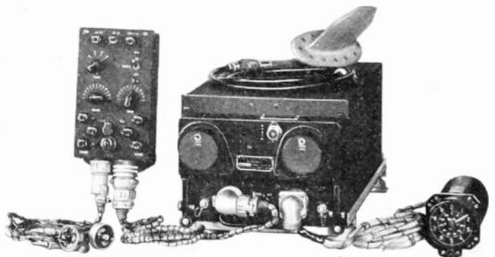
Fig. 2—Airborne pulse-multiplex DME showing control box, interrogator-respondor, antenna, and distance indicator.
