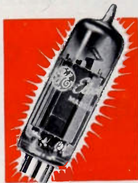
G-E receiving tubes of advanced design spell progress and economy. The new 6BN6, a miniature gated-beam tube, functions as a limiter, discriminator, and audio-amplifier in TV and FM receivers, thereby replacing 3 tubes and associated components.
