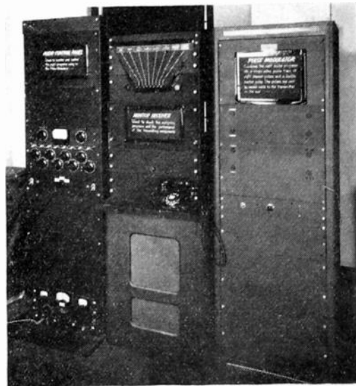
Fig. 2—Experimental multiplex broadcasting system, showing af control panel, pulse modulator, and monitor receiver.
