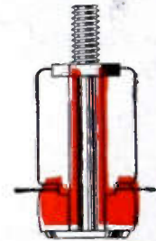
Silicone gaskets and porcelain stand-offs used with capacitors rated 2500-v to 5000-v d-c.
