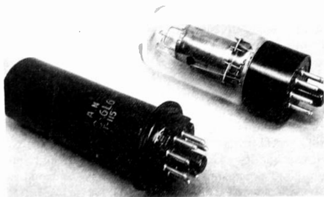
Fig. 14—Single-channel Cyclophon compared with a 6L6 metal receiving tube.
