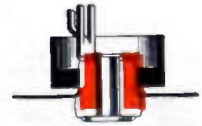
Silicone bushings and plastic cups used with capacitors 660-v a-c, or 1500-v d-c and lower.
