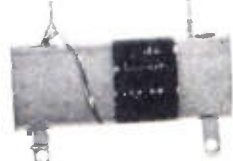
Hi Q oscillator coil — made to close tolerances mounts directly on band switch.
