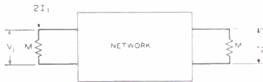
Fig. 6—Network connect to a source of admittance M at the input end, in 1 to a load of admittance M at the output end.
