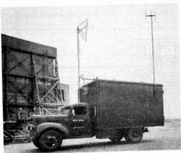
Fig. 4—Ground-speed-meter truck installation.
