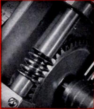
This 50-to-1 worm drive, equipped with a 3½ inch dial, is used for the fine setting adjustment. Backlash in the drive is kept very low by cutting the worm and its shaft from an integral steel shafting, eliminating eccentricity due to setscrews and misfit.
