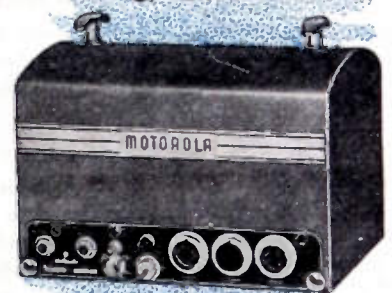
5516's power both driver-doubler and final of Motorola's Model FMTRU-30D.
