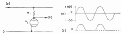
Fig. 2—A diode amplitude selector. Positive excursions of sinusoidal wave (a) exceeding the cathode potential of diode V_1 are selected as indicated in (b). Approximately ideal operation is obtained for input amplitudes of a few hundred volts.
