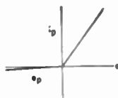
Fig. 1—The ideal broken-line characteristic of a diode.
