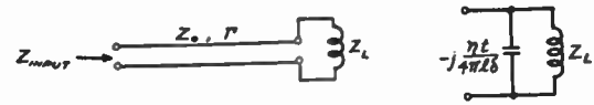
Fig. 3—Exact and simplified circuits for low-impedance gaps when Z_L \gg 2\pi l Z_0' / \lambda .
