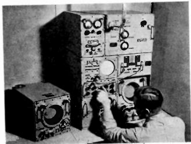
Fig. 5—The main rack and remote PPI of the RXF/268.
