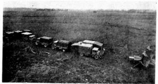
Fig. 12—Mobile ground-control-interception set: the RWM convoy deployed for operation. The radar antennas are in the right foreground with the IFF antenna in the background.
