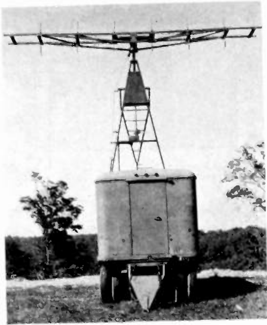
Fig. 4—Zone-position-indicator (ZPI) unit of the GL III C, taken at Leaside in early 1942.
