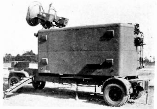
Fig. 3—Accurate-position-finder (APF) unit of the GL III C, taken at Leaside in early 1942.
