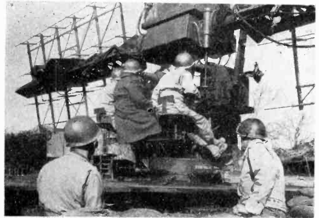
Fig. 24—Radio set SCR-268 in action at Nettuno, Italy, assisting anti-aircraft guns to shoot down German night bombers over the Anzio beachhead in 1944.
