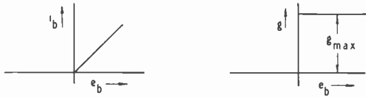
Fig. 3—Plate-current and conductance characteristics of idealized diode.
