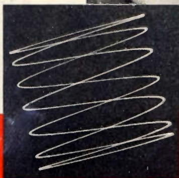
Trace showing absence of astigmatism. Frequency—60 x 420 cycles.
