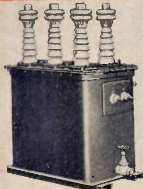
300 VA Filament transformer, single phase, 60 cycles, 6 secondary windings of 5 volts each; 3 secondary windings operating 40 KV above ground and 3 secondaries operating 20 KV above ground.
