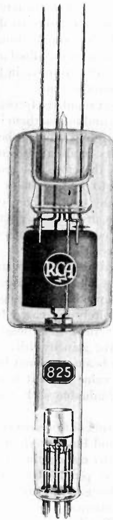
(Courtesy of RCA Victor Division of Radio Corporation of America) Fig. 20—Commercial form of the inductive output tube.
