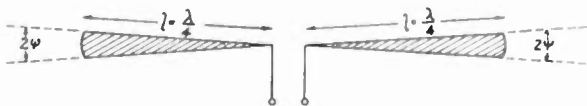
Fig. 5—A half-wave dipole formed by two conical conductors of apex angle 2\psi . Such a biconical dipole presents a uniform surge impedance to waves traveling along the length of the conductors.
