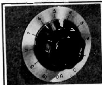
The attenuator gives the amplitude of the harmonic voltage directly in decibels below the fundamental.
