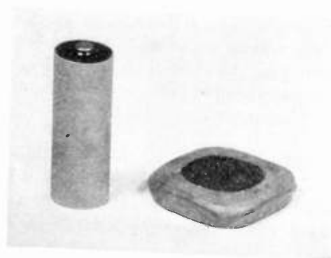
Fig. 12—Comparison between cylindrical and new wrapped type of flat cell.
