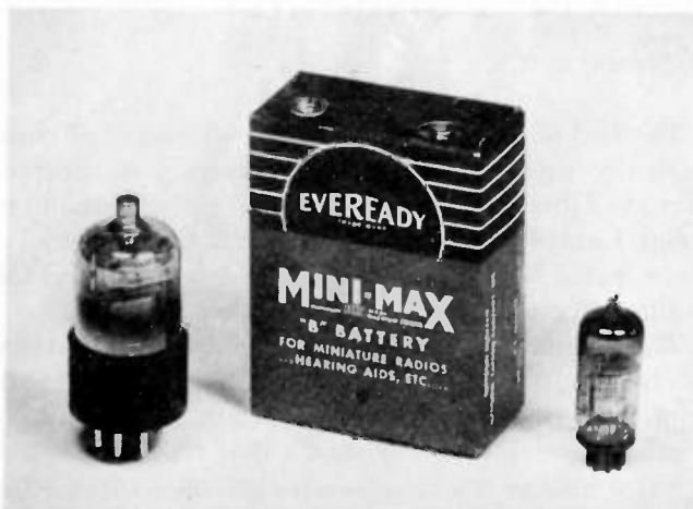
Fig. 2—New type 67.5-volt B battery for personal receivers.
