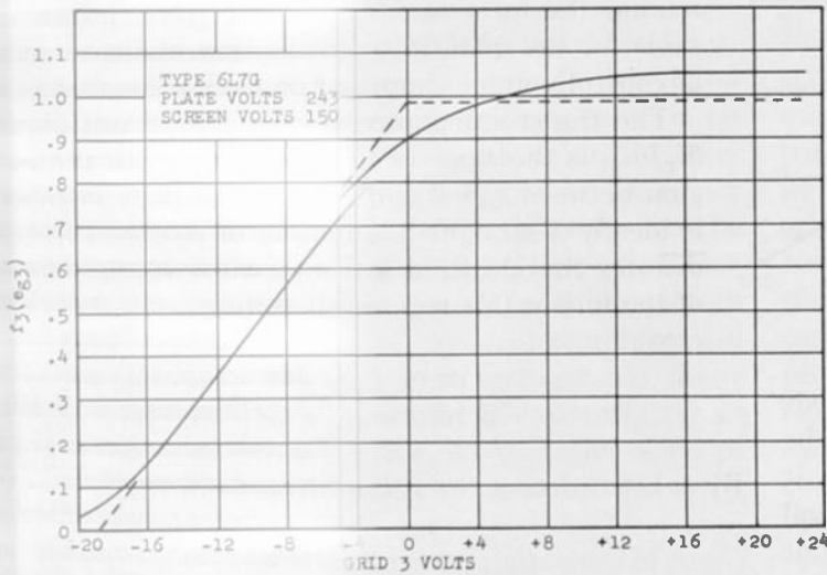
Fig. 3—Plate current as a function of grid-3 voltage expressed in terms of value at E_{c3} = +6 volts.
