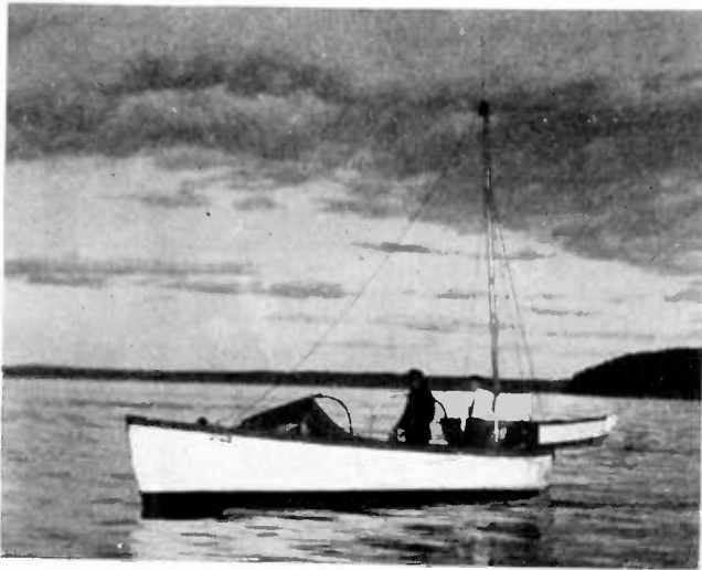
Fig. 6—Boat carrying measuring equipment. Receiver located in bow. Antenna shown in vertical position on rotatable wheel at top of mast.
