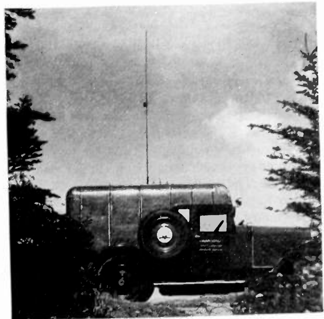
Fig. 5—Transmitter truck in location on Mount Cadillac. 55-megacycle vertical antenna in place.
