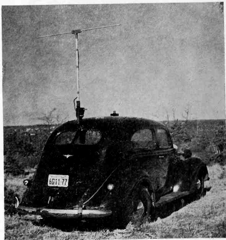
Fig. 1—Mobile field-strength survey car.
