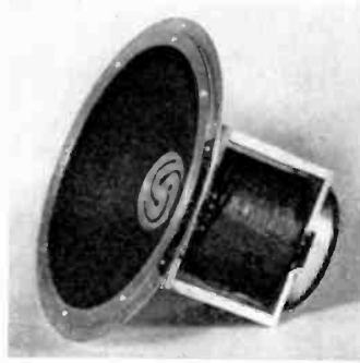
Fig. 9—Speaker mechanism employing two separate diaphragms mounted on a common magnetic structure. The low-frequency diaphragm is visible and the high-frequency diaphragm is mounted within the cylindrical enclosure at the right.
