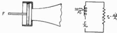
Fig. 1—Simplified horn loud speaker and equivalent electric circuit of the acoustic system.
