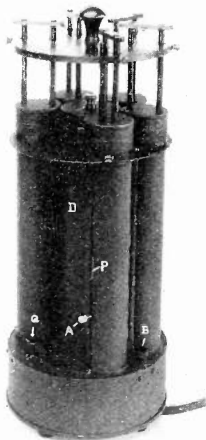
Fig. 3—A four-stage concentric-line tuned radio receiver for 175 megacycles (1.71 meters) to 300 megacycles (one meter).
