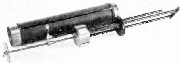
Fig. 5—One of the concentric lines showing tuning plunger and sliding antenna input terminal.
