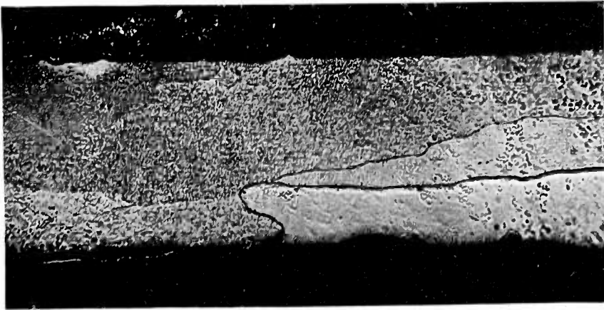
Fig. 2—Appearance of nonsag tungsten wire after burning, showing formation of long interlocking crystals which prevents wire from sagging.
