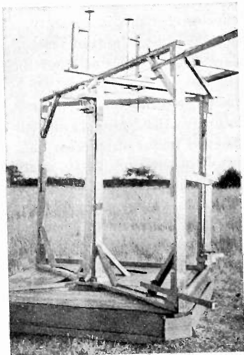
Fig. 4—Close-up of transmitter structure showing single wire reflector. The main antenna is on the left.
