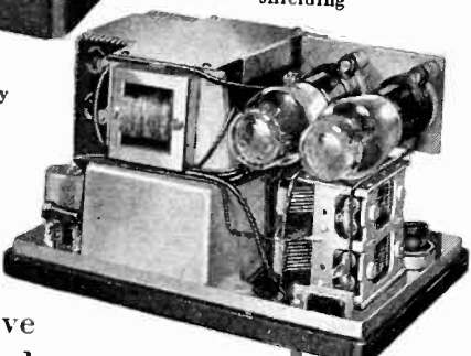
View showing chassis assembled and wired, without enclosing brass case
