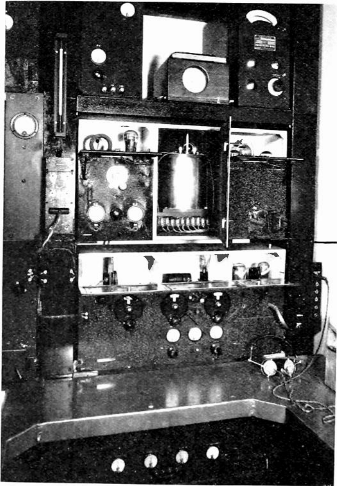
Fig. 10—Frequency standard—Rocky Point station. The oscillator and receiver units with doors open. In the central compartment of the oscillator unit is the thermal tank containing the crystal, in the left is the oscillator circuit, and in the right, the temperature control equipment.
