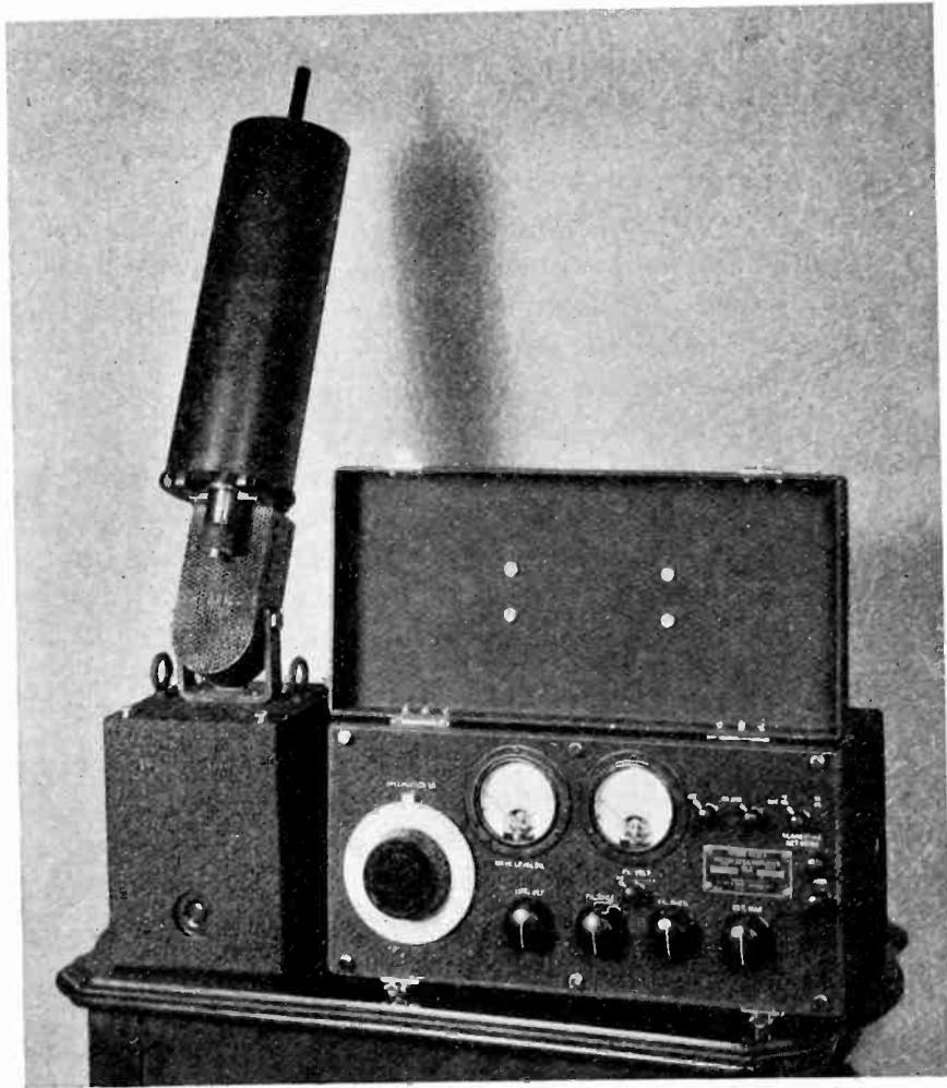
Fig. 1—Sound meter showing acoustical calibrator.
