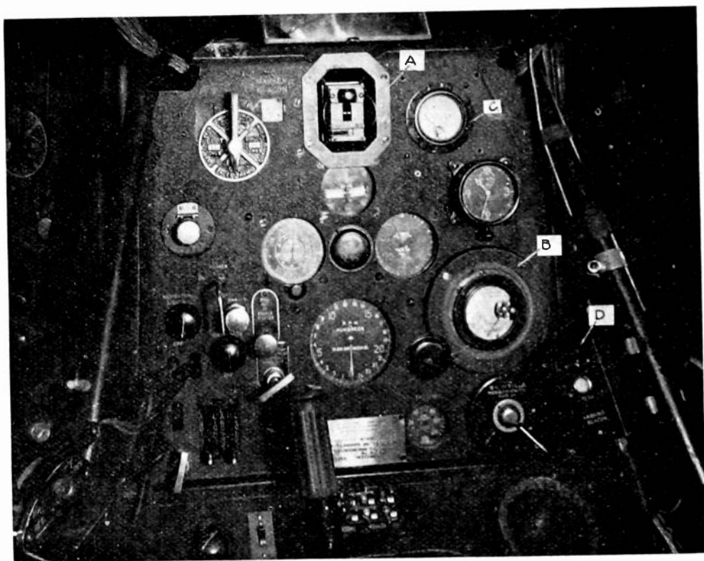
Fig. 12—Instrument board on Bureau of Standards' experimental airplane, showing vibrating reed course indicator A , landing beam indicator B , rough distance indicator C , and landing beam runway set control and test panel D .
