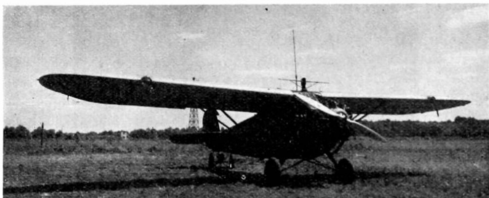
Fig. 8—Bureau of Standards' experimental airplane showing horizontal doublet antenna used for receiving the landing beam signals.
