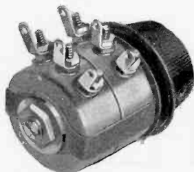
No. 590-590. Metal shell, composition element only. Resistances from 5,000 ohms to 1 megohm. All curves. Potentiometer or rheostat types. Units insulated from each other. Diameter, 1 5/16 in. Depth of shell, 1 1/8 in.
