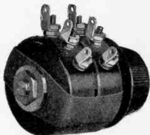
No. 2880-2880. Bakelite shell composition element only. Resistance range from 5,000 ohms to 1 megohm. All curves. Potentiometer or rheostat types. Units insulated from each other. Diameter, 1 1/2 in. Depth of shell, 1 1/8 in.
