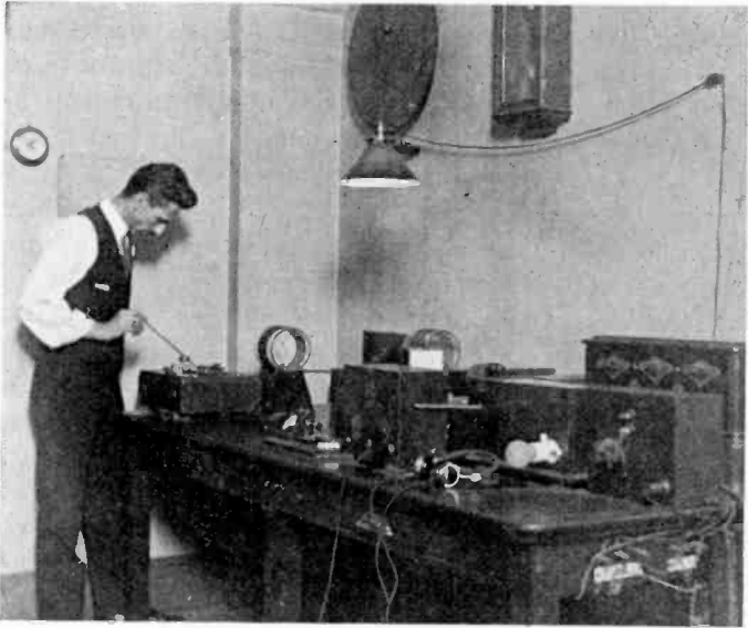
Fig. 1—View of Measurement Apparatus Employed for Checking the Operating Frequency of Broadcast Stations.
